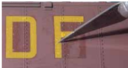
Fig. 5 AIR BUBBLES. Trapped pockets of air show up as raised bubbles (at the point of the knife) or silvery areas (on the right of the F). Prick them with a knife.
