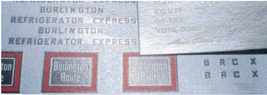
Fig. 3 DECAL FILM. Microscale decals (at left) have decal film only under the lettering and graphics. Other brands, such as Champ (right), have film on the entire sheet.
