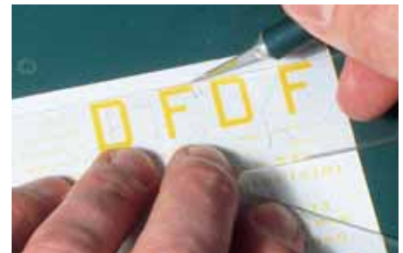
Fig. 2 CUTTING DECALS. A clear drafting triangle works well for guiding the blade, and a self-healing cutting mat is a good surface.
