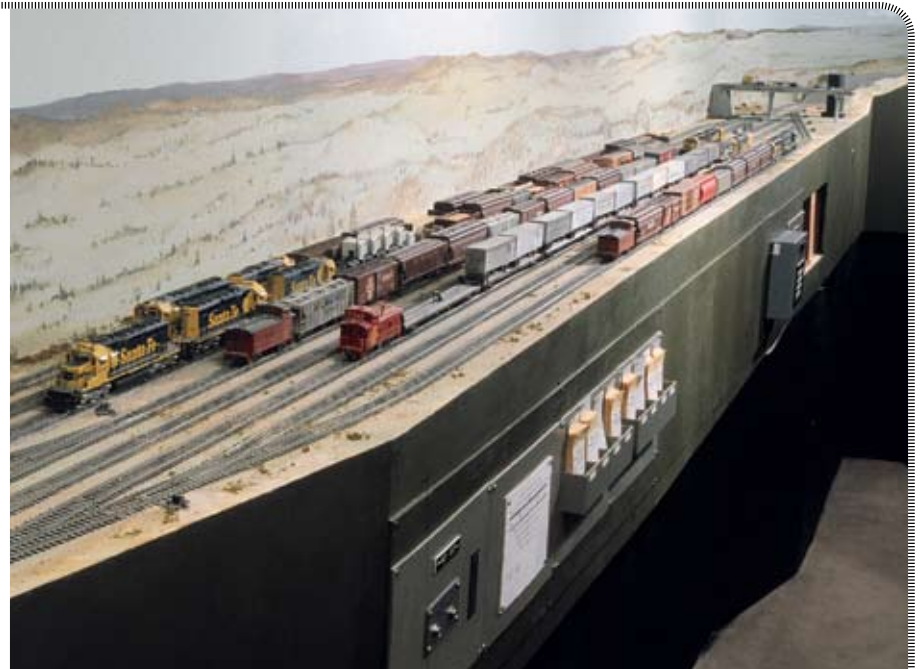
David Barrow, a proponent of open staging, built this double-ended open staging yard on his HO Cat Mountain & Santa Fe Ry. The near end represents the east end of the line as East Hill. The other end is called West Mesa to represent the western end of the railroad. Tommy Holt photo
