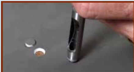
**I made manhole covers** by using a 1/4" leather punch to pop holes into the .080" styrene streets, taking care to save the inserts. I used the jaws of my bench vise to press a cross-hatched pattern into these inserts. After painting the holes with a black marker, I used a small brush to lightly dust the covers with Polly Scale CP Gray.
