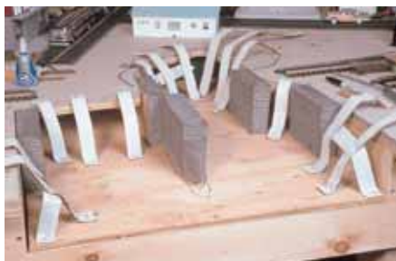
Fig. 3: Once the abutments are in place, you can cut cardboard strips shaped to the rough outline of the walls of the gorge and staple them in place.
