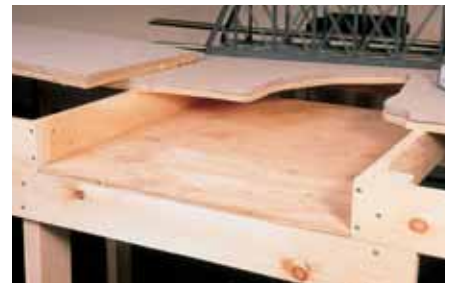
Fig. 2: Next frame the gorge with 1-by-4 sides and a base made of plywood. Be sure that the pieces of wood fit flush to the front edge of the layout.
