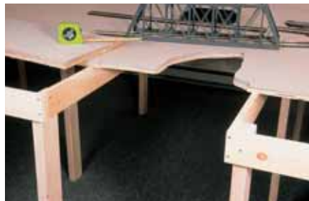
Fig. 1: Start by cutting out the shape of the gorge and any underlying braces. The width of the cut in the tabletop is a couple of inches less than the bridge that spans it.
