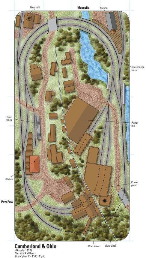
**Cumberland & Ohio** HO scale (1:87.1) Plan size: 4 x 8 feet Size of plan: 1° = 1'-0°, 12° grid Illustration by Jay Smith Find more plans online in the ModelRailroader.com Track Plan Database © 2012 Kalmbach Publishing Co., Model Railroader magazine. This material may not be reproduced in any form without permission from the publisher.
