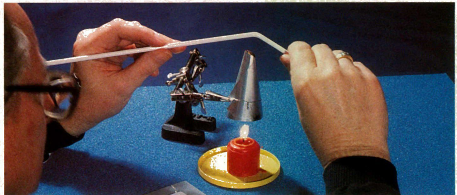
Fig. 4. BENDING THE TUBING. Concentrating the heat from a candle with material from an aluminum can makes it easy to bend the Plastruct tubing.
