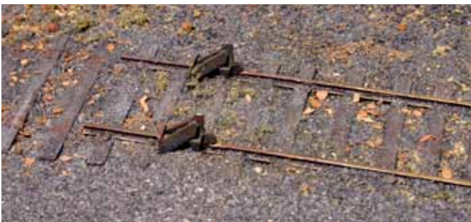
Used in pairs and often found on industrial spurs, wheel stops keep cars from rolling off the end of the line. These Tomar Industries HO castings model a Hayes design.
