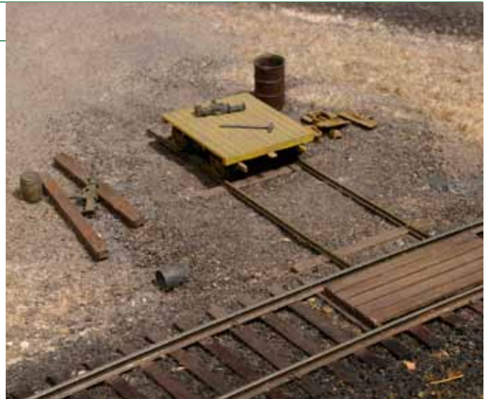
Handcar setouts use wooden beams or rails installed perpendicular to the track. A pile of ballast or a wooden platform makes it easier for the handcar or motorized speeder to be rotated onto the setout and out of the way.
