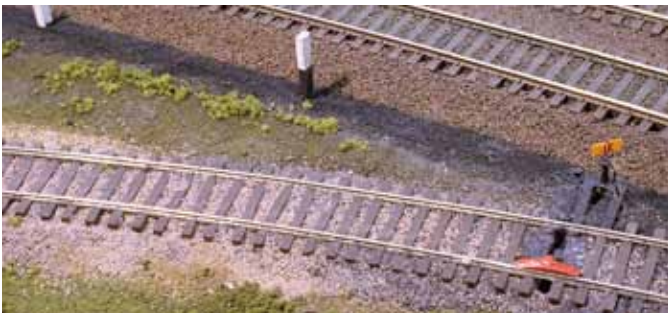
Derails are often used at sidings to keep a runaway car from fouling the main line. Bill Aldrich modified this HO hinged-block derail to actually operate via a switch stand.
