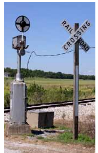
Wig-wag signals, such as this one on a former Atchison, Topeka & Santa Fe line in Cherryvale, Kan., have a swinging head that simulates the motion of a brakeman's lantern.
