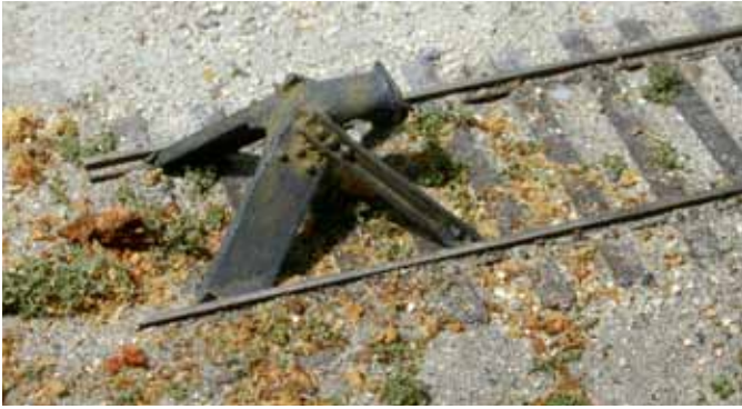
A few manufacturers sold their own distinctive bumping posts. This HO scale casting from Custom Finishing depicts a Durable Model D bumping post.
