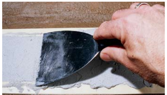
Fig. 1 Finishing the surface. Lou Sassi uses a putty knife to smooth Concrete Patch, a modeling material similar to spackling compound, between the masking tape forms.
