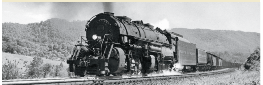
Sand on the rails and the smoke plume from the class Y6b 2-8-8-2 show what hard work was required to lift Norfolk & Western coal trains up the 1.2 percent Blue Ridge Grade at Blue Ridge, Va. Tom Miller photo
