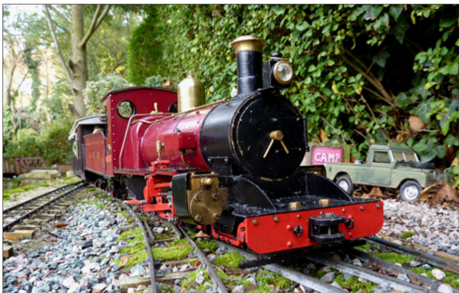
4. Siliguri , a Darjeeling C class Pacific, is the largest engine on the line. It is coal fired and was built by Mike Gaskin.
