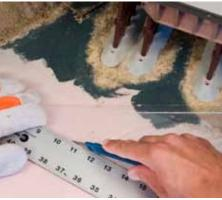
2 Position the acrylic panel over the scene to determine what needs to be trimmed. Use a plastic-cutting knife to first score the panel, and then cut or snap the panel to fit. Use a straightedge and clamps to ensure safe cuts.
