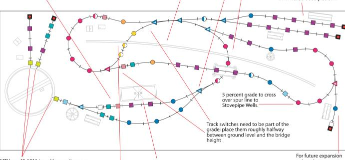
MTH no. 40-1011 transition sections are shown here, but you may be able to skip the transition pieces by cutting off RealTrax pins and clips and carefully aligning sections to meet the Atlas O rails on the turntable
