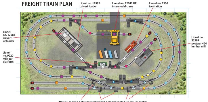
Narrow spacing between tracks won't accommodate Lionel O-72 switch machines. Try using Ross Custom Switches' new RossPlate track switches with traditional tubular rail and small no. DZ-2500 switch motors
