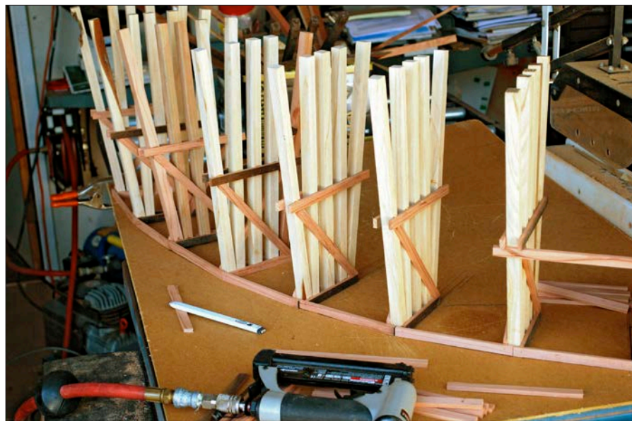
5. The trestle being assembled upside down. Bents are equally spaced and connected at their outside edges.
