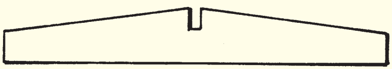
roof beam cut 4 from 1/8" stock
