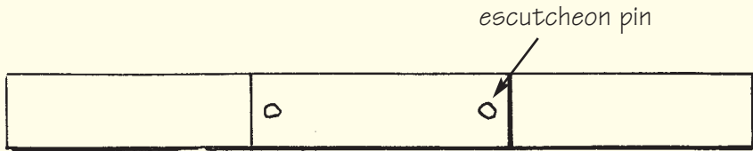
end beam make 2 from 1/4" x 7/16"
