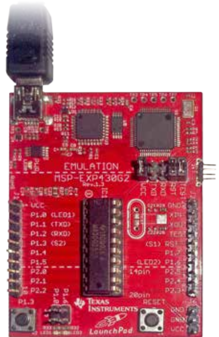
1. The Launch Pad is connected to any Windows computer via a USB cable for programming.
