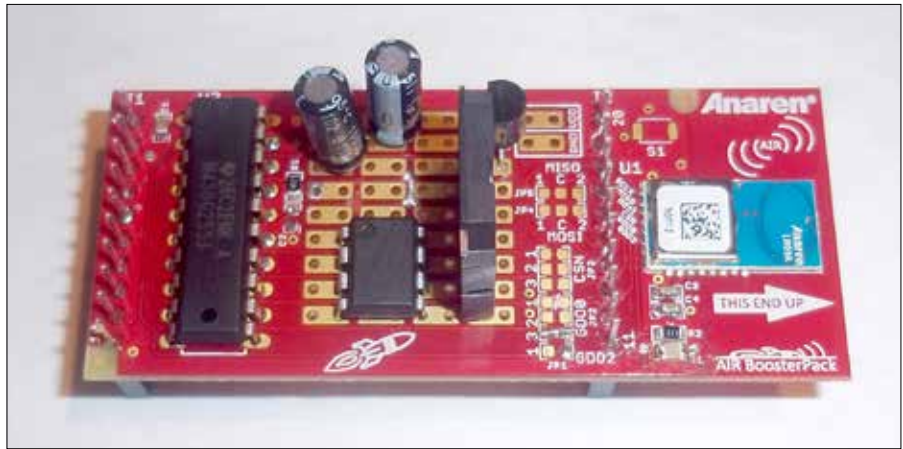
6. The PCB with the ICs and capacitors in place.
