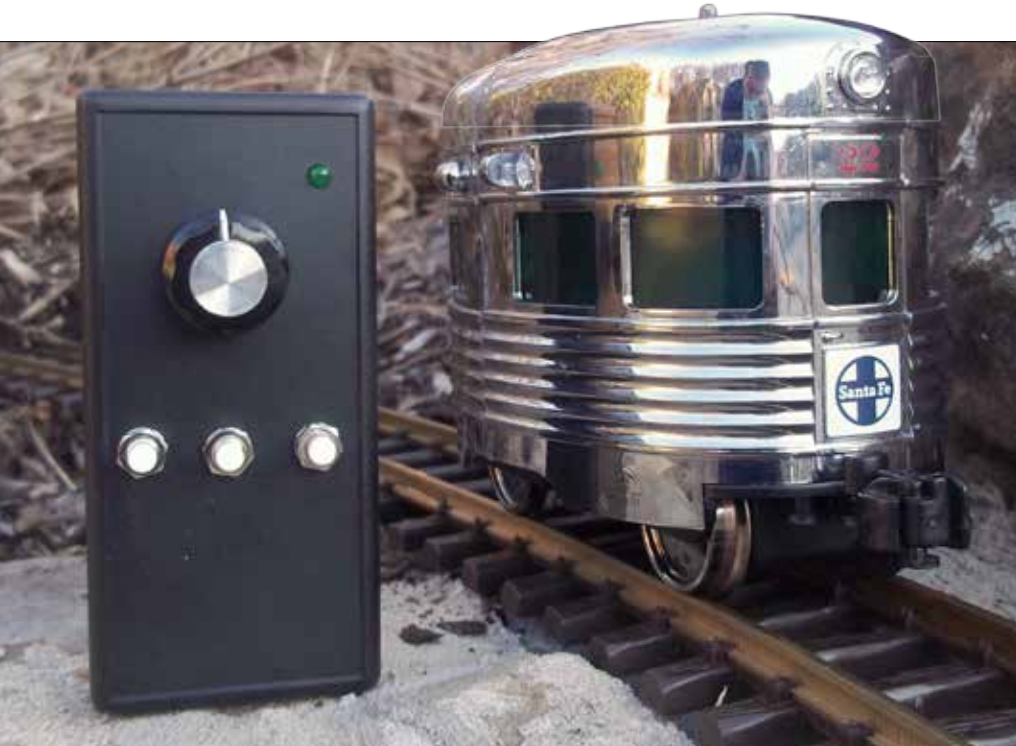
The Junior Operator DCC throttle (left) is a basic unit that anyone can build at low cost.
