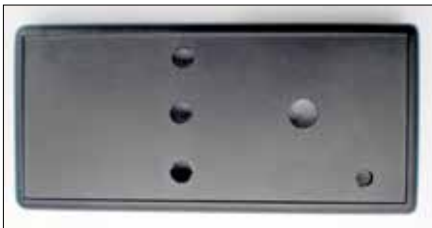
10. Holes have been drilled in the enclosure using the drill template as a guide.
