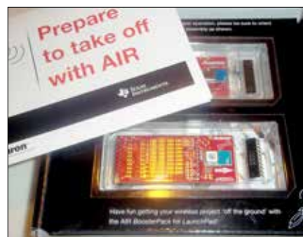
2. The Anaren "430BOOST-AIR Booster Pack" kit is the heart of this project.
