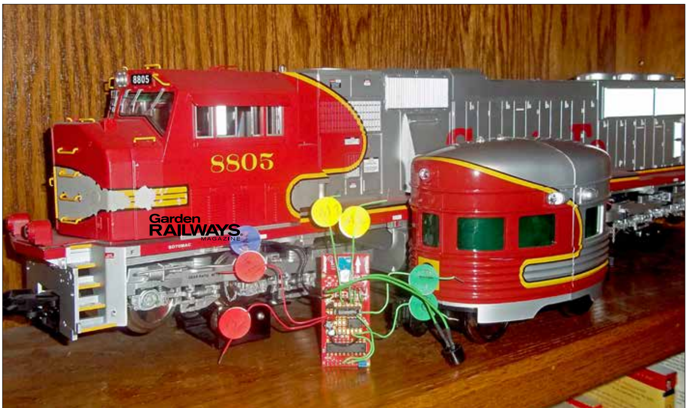
1. The DCC decoder, ready to be installed in your locomotive of choice.
