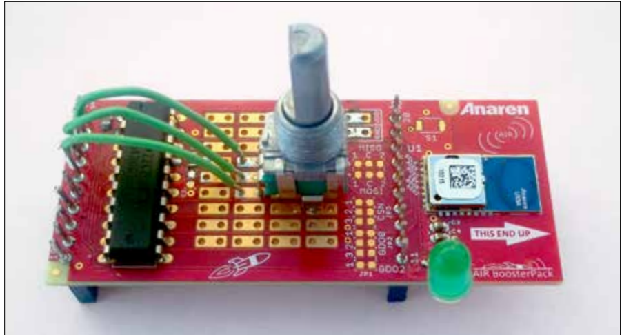
7. The potentiometer and the new leads installed on the board.
