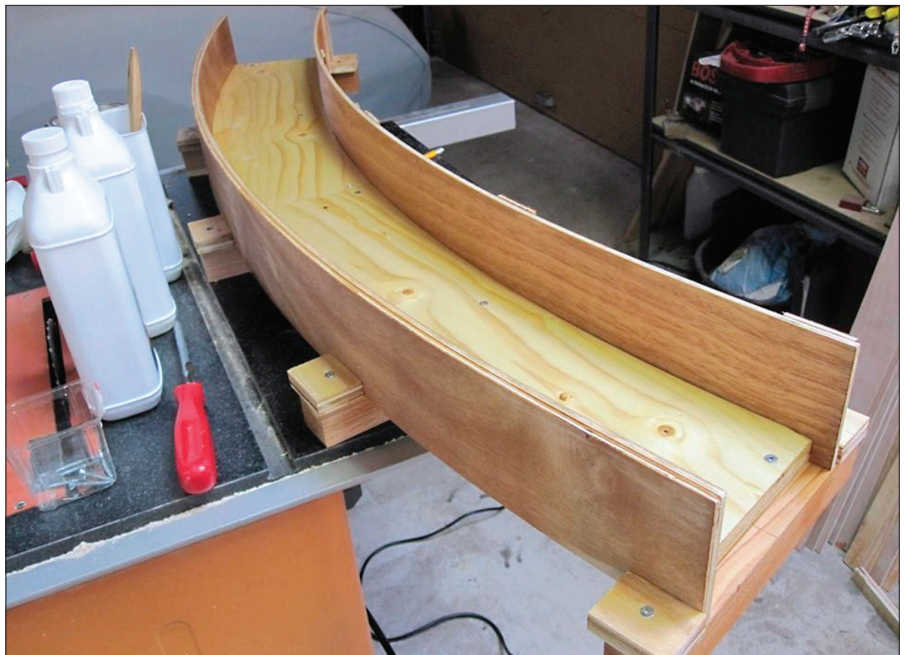
8. The finished sides are nicely curved. Form walls are held in place with wall retainers, screwed to the feet below.
