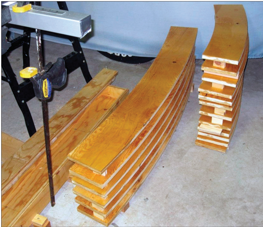
5. All of the bases have been treated with urethane to make them moisture resistant.
