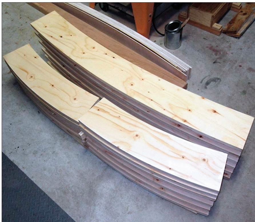
4. Plywood form bases for 5'- and 10'-radius track.
