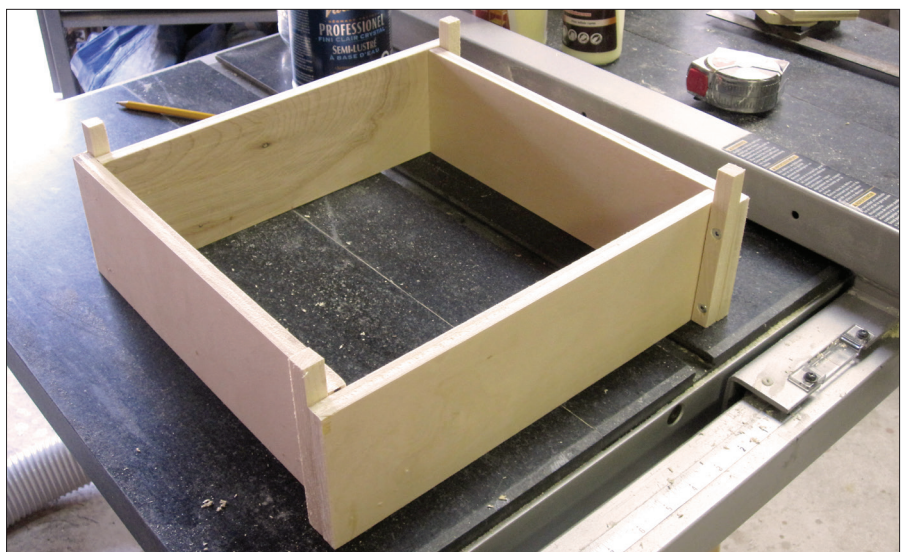
9. Forms for the footings are made from four pieces.
