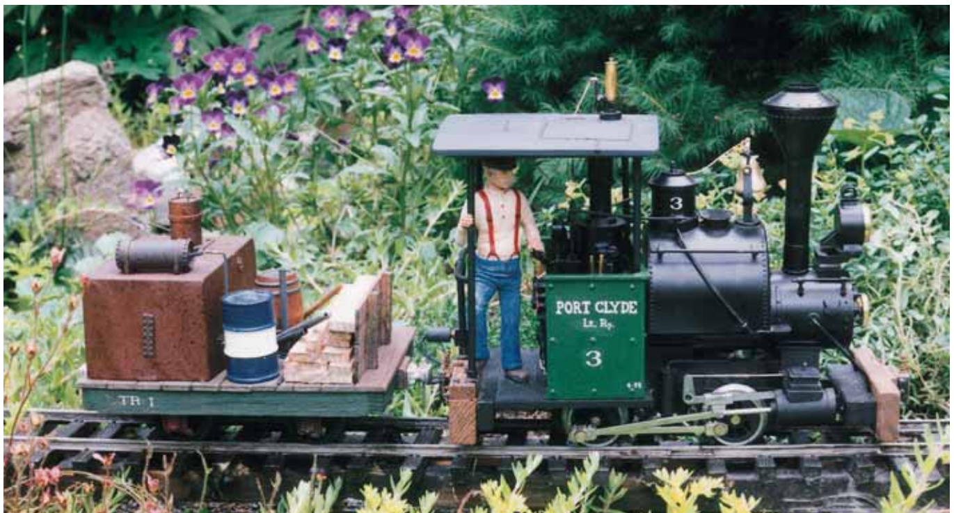
BELOW: Port Clyde No. 3, a heavily kitbashed Lehmann locomotive, tows a supply car that houses the batteries that power the engine. The author made the engineer from polymer clay.
