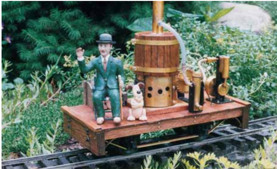
LEFT: A \frac{7}{8} " scale, live-steam locomotive based on a Midwest marine steam plant. This engine is typical of a homemade, backwoods locomotive.
