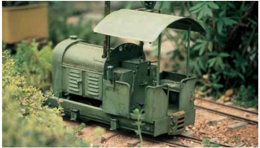
Arthur is a battery-powered, scratchbuilt locomotive on the 18"-gauge Excelsior Estate Ry. The locomotive is constructed almost entirely of brass. Careful weathering and attention to detail give this engine veracity.
