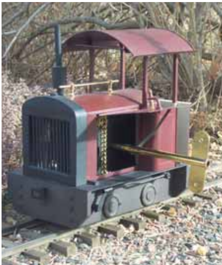
While exceedingly uncommon, clockwork engines can be a lot of fun. This one was built by Marc Horovitz in 7/8" scale, using a Meccano clockwork motor.
