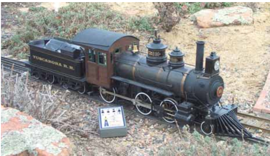
Radio control frees you from the vagaries of track power, but the R/C system must be purchased separately and installed, as it was in this engine.
