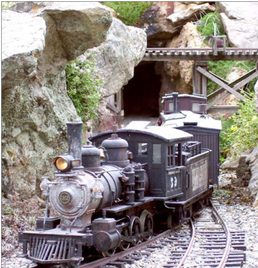
3. Engine N° 39 is a battery-powered Delton C-16 Consolidation with SoundTraxx Sierra sound. The NiMH batteries, installed by Battery Back-Shop, will pull a short freight around the line for up to two hours before recharging.
