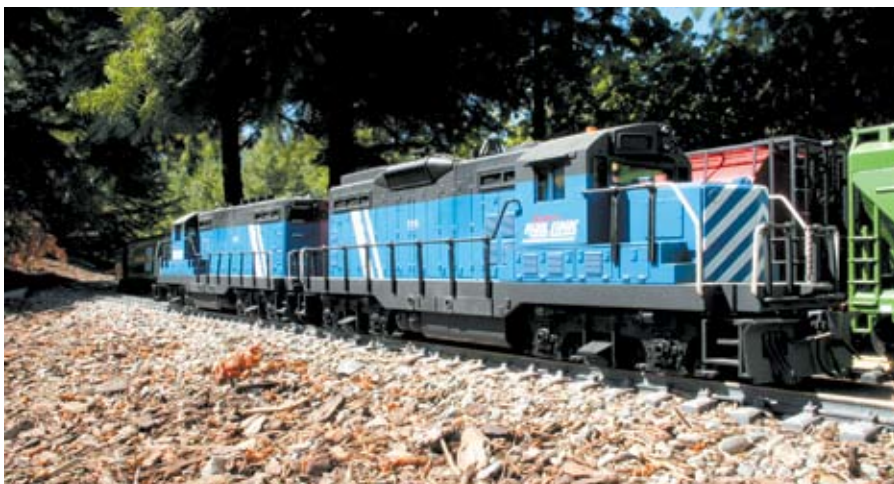
5. Grant Minor, a friend of and collaborator with the author, heavily rebuilt these Lionel GP20s. The pilots and almost all of the roof details were scratchbuilt.
