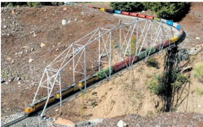
7. The steel truss bridge spans a deep gully. It was assembled entirely with screws and nuts on a purpose-built table.
