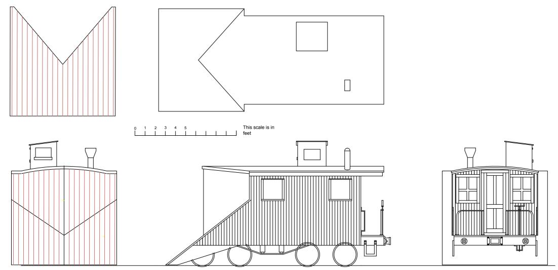
The spacing of the wheels is based on Bachmann trucks.
