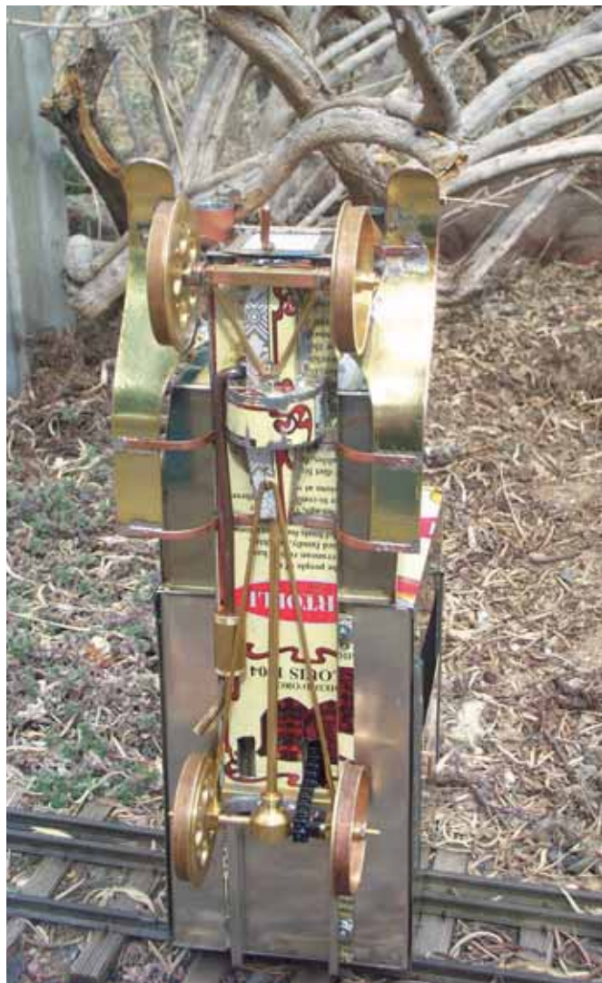
The underbody detail was supposed to be made of wooden shapes (according to the plan), but ended up here rendered in tinplate. The differential was turned on a lathe.
