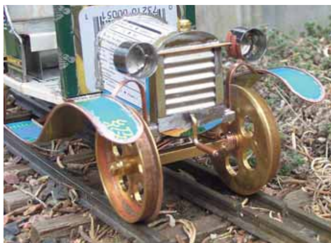
The grill was made by running a piece of tinplate through a tube squeezer. Headlights were rolled around a dowel and soldered. Non-working leaf springs were made from flat wire.
