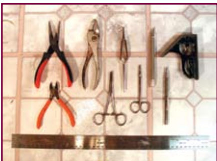
Some of the more common hand tools found around the workbench. Top row (left to right): Needle-nose pliers, standard pliers, tweezers, X-act knife, and square. Middle row: Diagonal cutters, hemostats, scissors, and scribe. Bottom row: 18" metal ruler.
