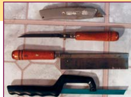
Cutting devices. Top to bottom: A box knife, small razor saw, large razor saw, and hacksaw.
