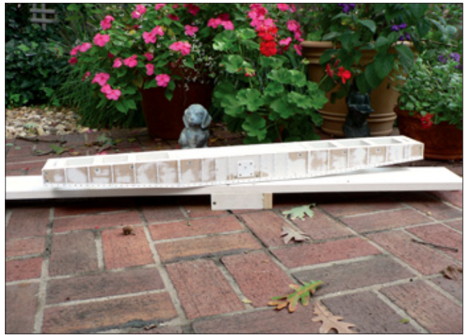
4. A 6" board forms the center of the base and houses the bearing.
