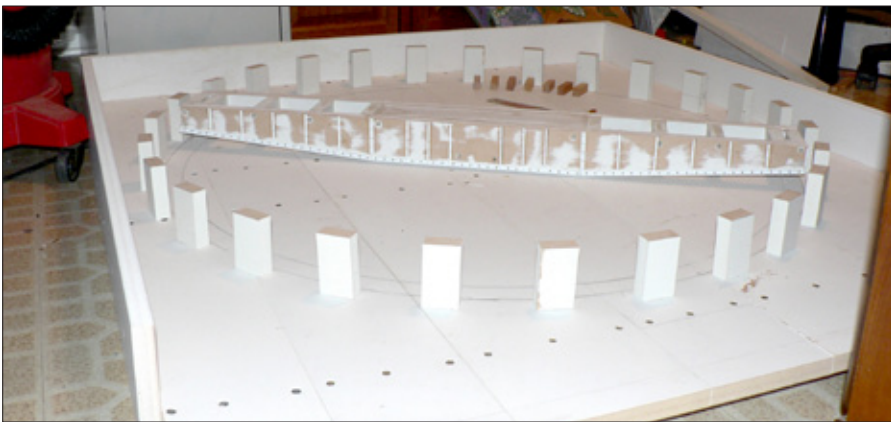
6. To form the pit wall, small pieces are screwed into place from underneath.
