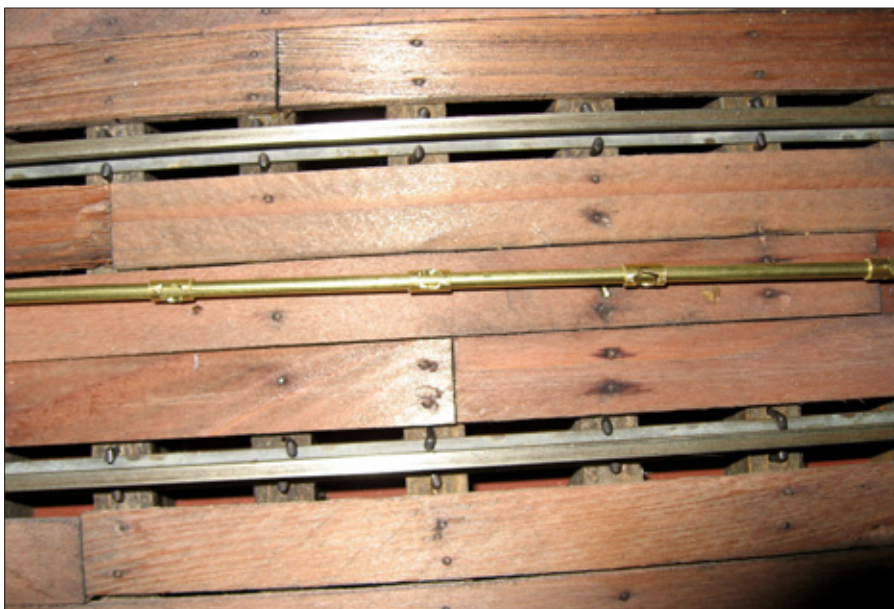
15. The top "T" sections have been slipped over the \frac{3}{32} " rod.
