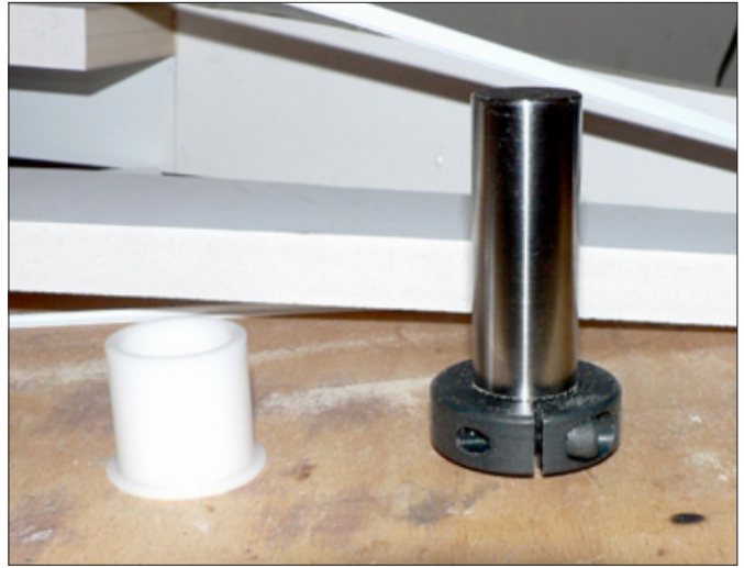
2. The turntable rides on a steel shaft and Delrin bearings.
