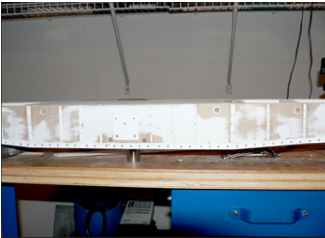
3. Rivet detail and a styrene cover over the access hole have been added.
