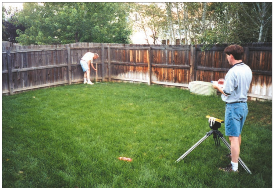
Surveying the railroad is best done by two people. Standing at the laser, I record the measurements that my father, holding the yardstick, calls out. Ruth Strong
