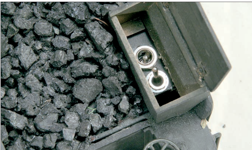
For nonremovable batteries, provision must be made for charging them. Here, the power switch shares a toolbox with the charging jack.
