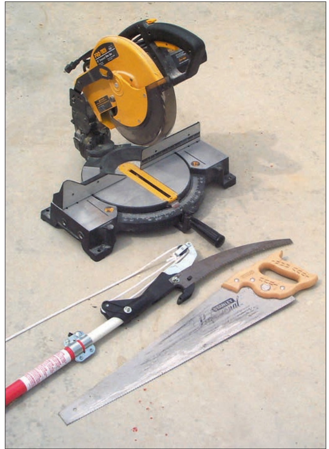
A power miter saw, handsaw, and tree saw handle many of the cutting tasks found in a garden railway.
