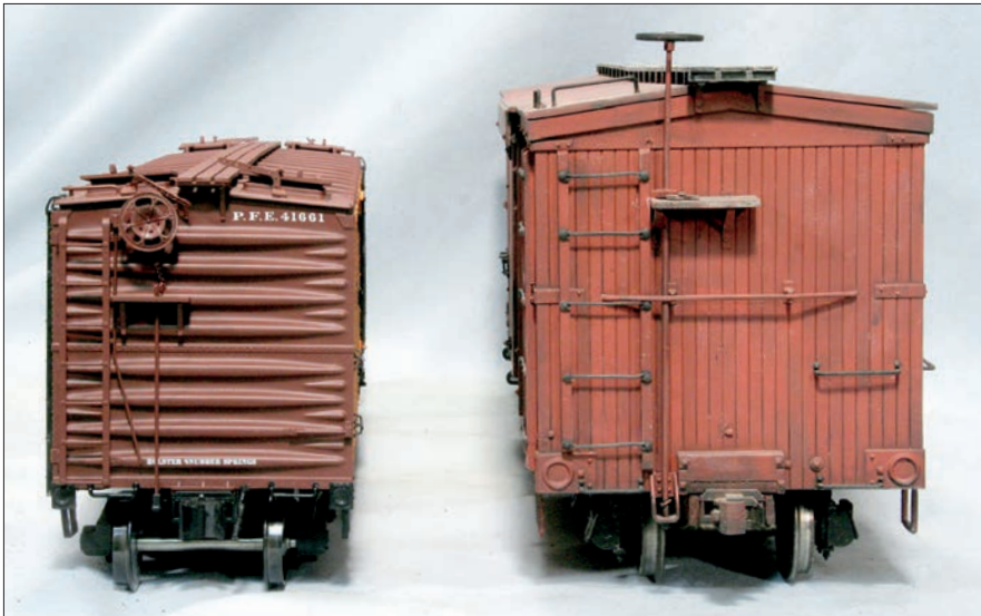
In large scale, where the track gauge is constant, the size of the equipment increases with the scale. Here, a 1:32 scale, standard gauge car (at left) is dwarfed by its 1:20.3 narrow gauge counterpart—essentially reversing the proportions in the prototype photo shown on page 13. There is no difference in track gauge.
