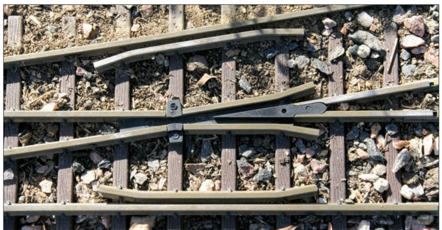
The frog and guardrail flangeways—like the points—need to be kept clear. These areas aren't quite as prone to debris jumping in during normal operations.
