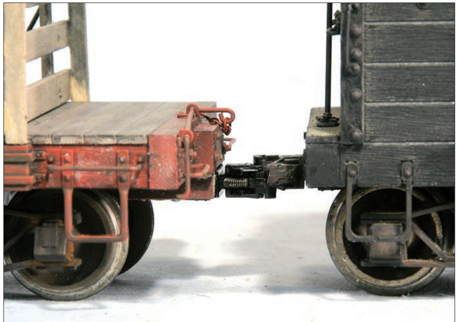
If a coupler sits too high or too low, it may uncouple on uneven track. The coupler on the left needs to be raised around 1/16 " to match the correct coupler.
