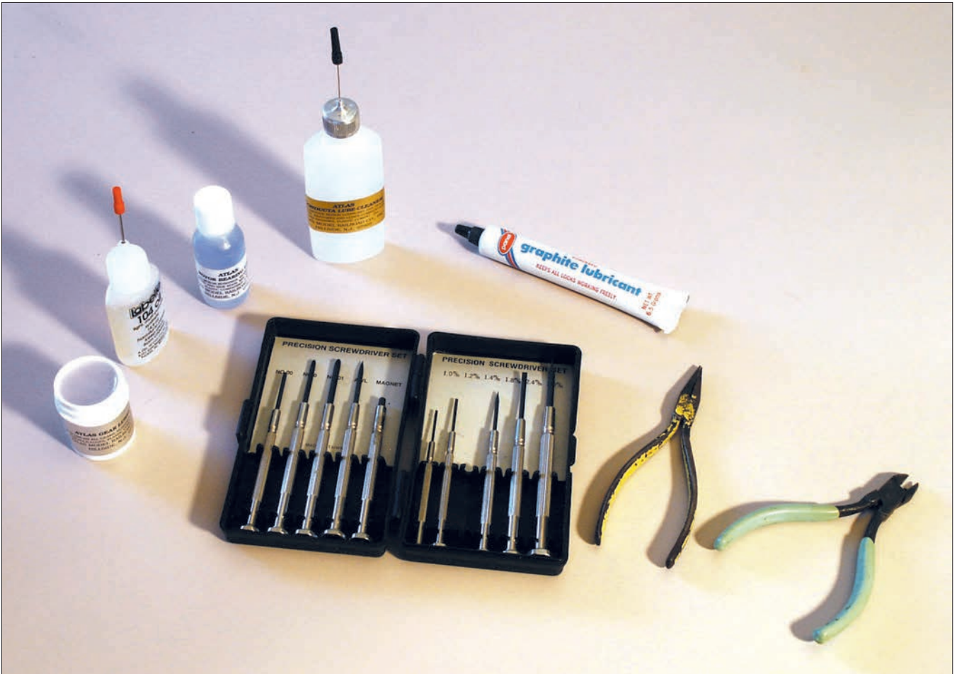
Maintenance tools should be in every modeler's toolbox. These can include (left to right) plastic-compatible gear grease, sewing machine oil, plastic-compatible bearing oil, conductive lubricant, powdered graphite (for couplers and other surfaces where oil is undesirable), a set of small jewelers screwdrivers (both Phillips and slotted), needlenose pliers, and diagonal wire cutters.
