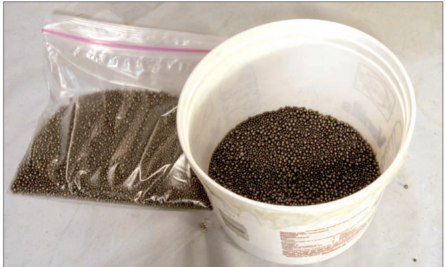
Lead shot makes a great weight for locomotives because of its ability to fill in any available space. It can be used in bags or mixed with putty or clay to take on a more solid form.
