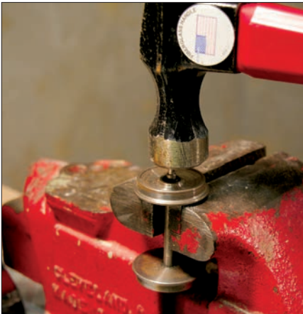
If the wheelset is gauged too narrow, a light tapping on the end of the axle will move the wheel out the desired amount.
