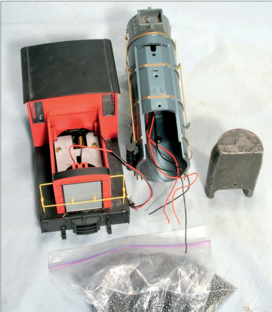
Typical locations for weights in large scale trains are shown here. Diesels usually have the weights on or near the floor of the locomotive. In this case, the frame is also metal, adding even more weight. Steamers typically have large metal weights inside their boilers.
