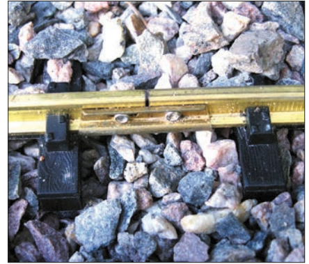
Screws through the rail joiners are perhaps the simplest method of maintaining a good connection between the rails.
