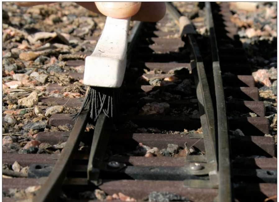
Keeping dirt and debris out of the moving points is imperative to proper operation. During operating sessions, I use a stiff brush to keep things moving freely.
