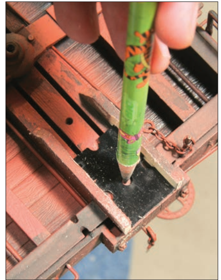
The coupler pocket is used to mark the location of the mounting holes to be drilled into the pad.
