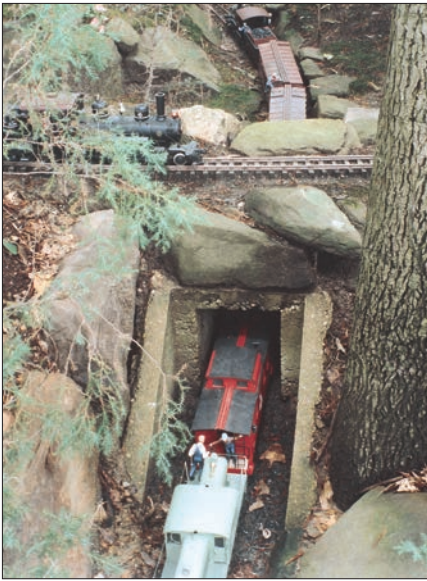
A train passing over another is dramatic, but you have to be careful of the steepness of the grade leading to the crossing. On this stretch of the Woodland Railway, the track passing through the hill is at a steep 5 percent grade. A helper locomotive on the rear of the train is a necessity.
