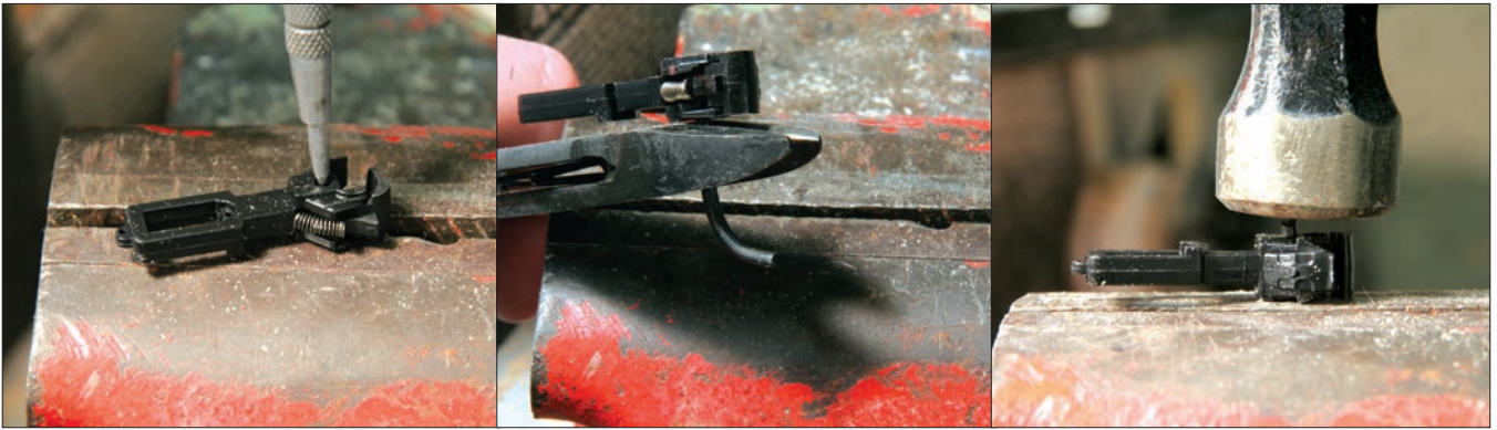
I cut the unsightly steel pins off of the couplers by (left) tapping the pin down around \frac{1}{16} ", (center) snipping off the pin, and (right) tapping the stub back into place. You'll know it's back in place when the knuckle opens and closes smoothly.
