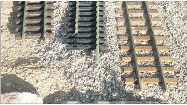
Three types of track are available in the garden. Sectional track (left) is perhaps the easiest to use. Flextrack (center) offers flexibility in planning and track design. Handlaid track (right) offers the highest level of realism, but it also requires the most planning and work.
