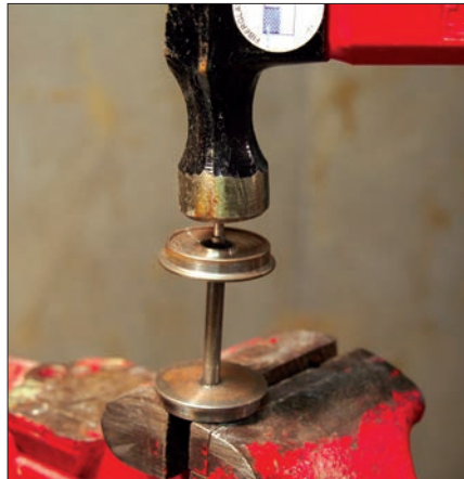
If the wheelset is gauged too wide, tapping the axle against the opposite wheel brings the two wheels closer together.
