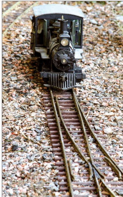
When an approaching train crosses the points first, it's a facing point because, from this direction, the switch determines which direction the train goes.
