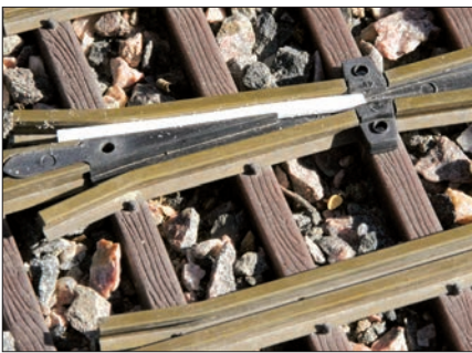
Deep flangeways can be filled with small strips of styrene to build up the base.
