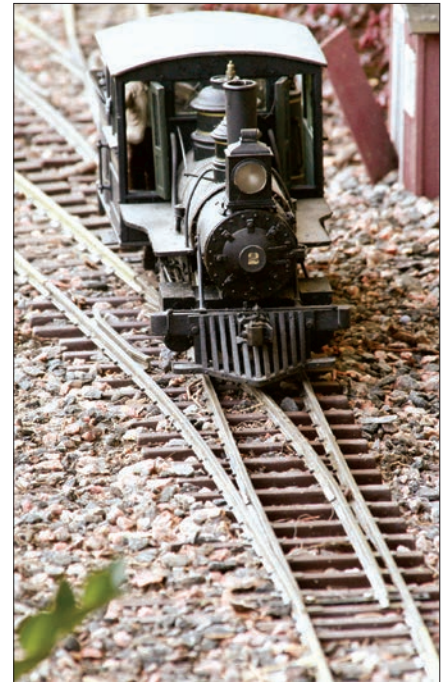
When a train passes over the frog first, it's a trailing point. Traveling in this direction, the switch brings the train into a single track. The points let it make this transition.
