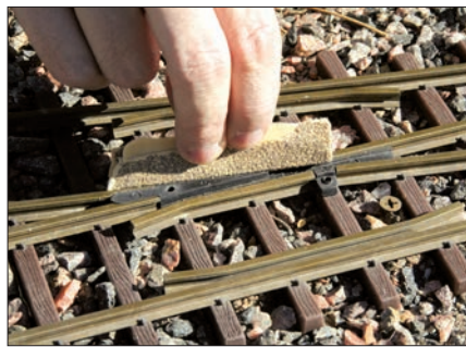
If the flangeways are too shallow, sanding and filing will remove excess material, so wheels can pass through without bumping.
