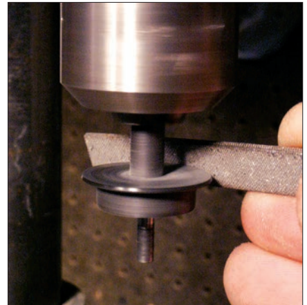
If the wheel can be removed from the car, then it may be possible to chuck it in a drill press to file down an oversized flange.
