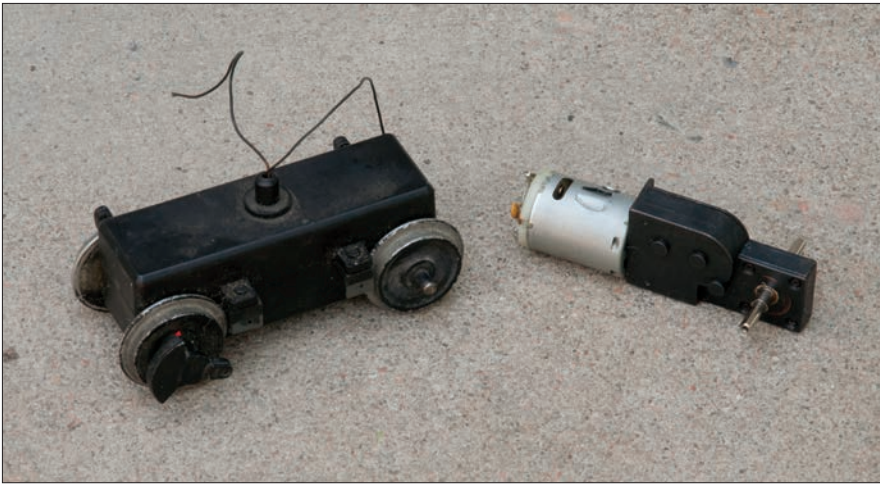
There are two common forms of motor and gear boxes in large scale. The enclosed box (on left) is common on diesels, though LGB and Hartland use them extensively on their steam locomotives as well. The motor and gear tower (right) is common on steam locomotives.
