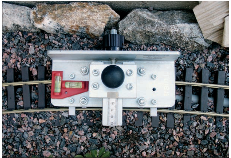
A dual-rail bender comes in very handy for bending rail that's already assembled onto tie strips. This one, by Train-Li, also has levels on it for checking the geometry of track that's already on the ground.
