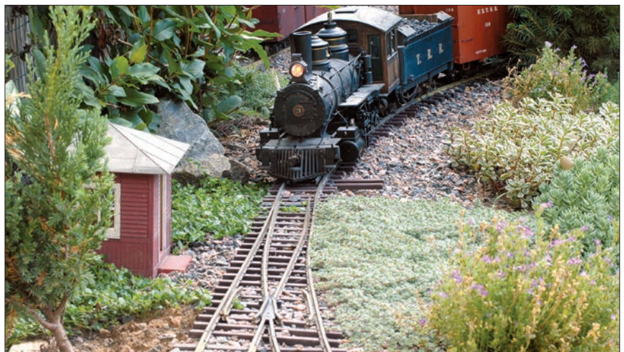
Tuscarora Railroad No. 3 pulls in to Shade Gap, passing over the switch that leads to the coal tippie. Switches are a vital part of railroading, both prototype and model. Without them, we'd be confined to running trains in a simple loop.
