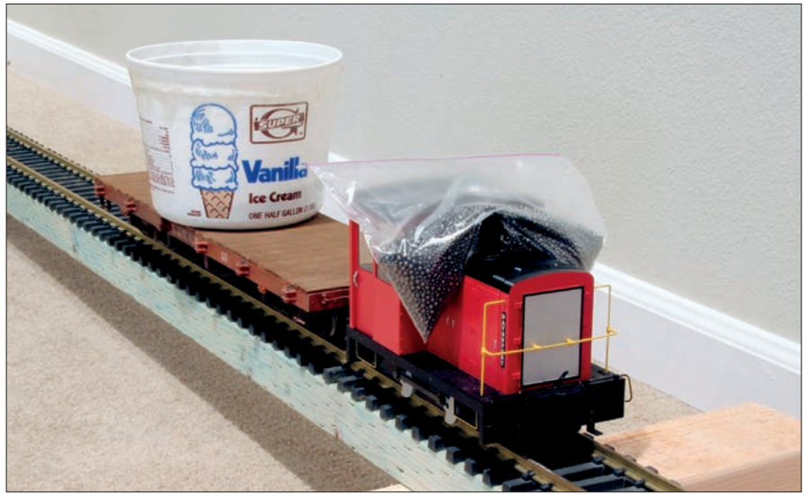
On my test track for adding weight, the 8'-piece of track is elevated about 4" at one end to create a 4 percent grade. The flatcar has a heavy load on it to simulate a longer train.
