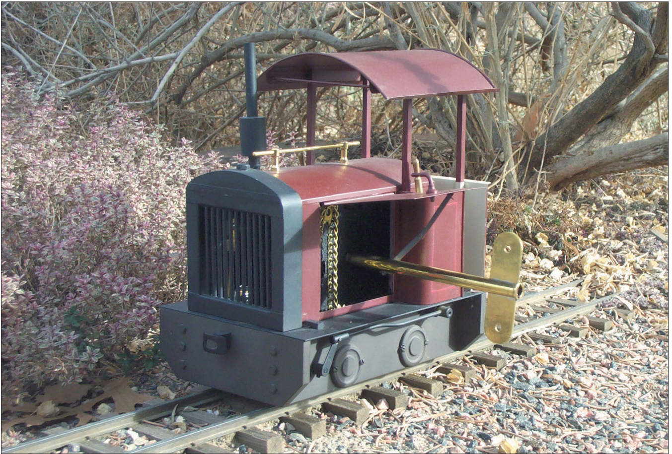
While exceedingly uncommon, clockwork engines can be a lot of fun. This one was built by Marc Horovitz in \frac{7}{8} scale using a Meccano clockwork motor. Marc Horovitz
