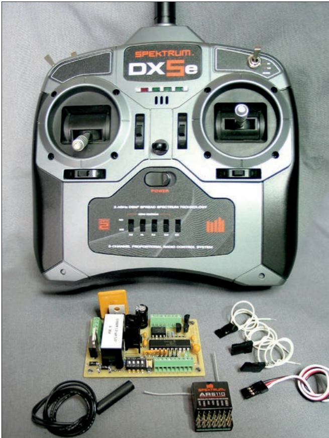
Some systems use commercial radio control gear and furnish an add-on throttle, such as G-Scale Graphics' RailBoss shown here and RCS's Beltrol systems. Any radio control controller will work with these throttles, but the throttles cannot be linked to other manufacturers' similar throttles for consisting or other purposes.
