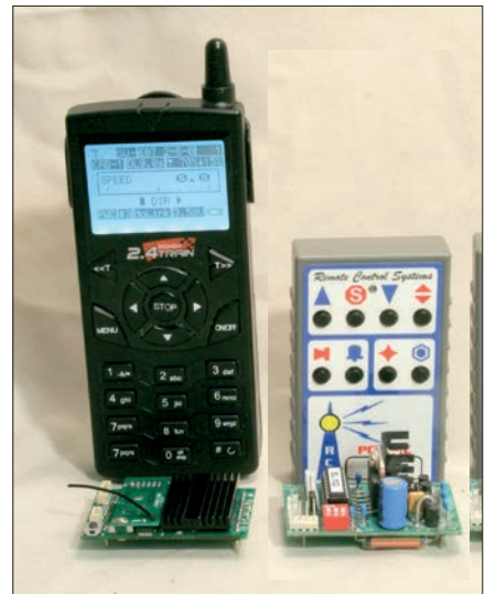
Proprietary systems include Aristo-Craft Revolution (left) and RCS Elite. There's no cross-compatibility between brands.
