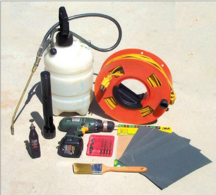
A cordless drill with screwdriver and drill bits and a Dremel motor tool are valuable tools for anywhere in the garden. If an extension cord is needed, make sure you have one that is long enough. A weed sprayer, paintbrush, and sandpaper help keep track clean.
