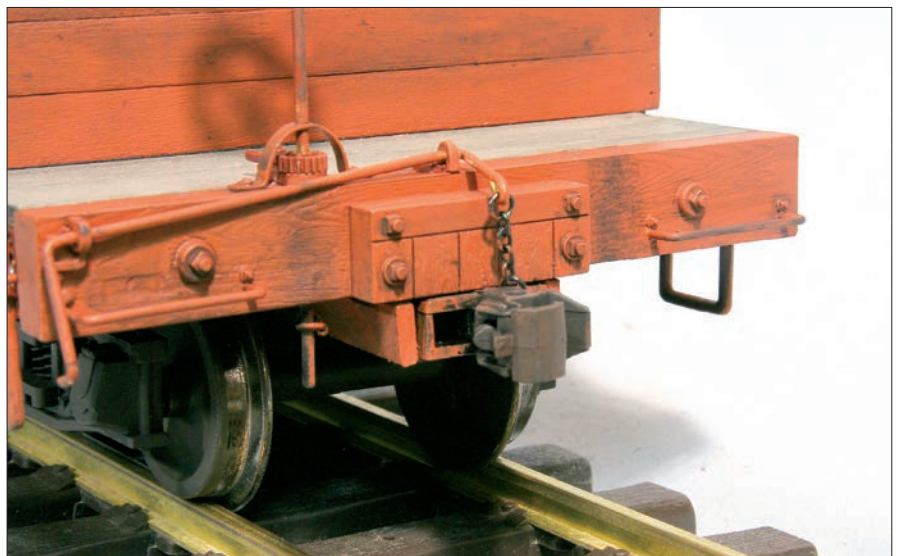
Body-mounted couplers are prototypically attached to the body of the car.
