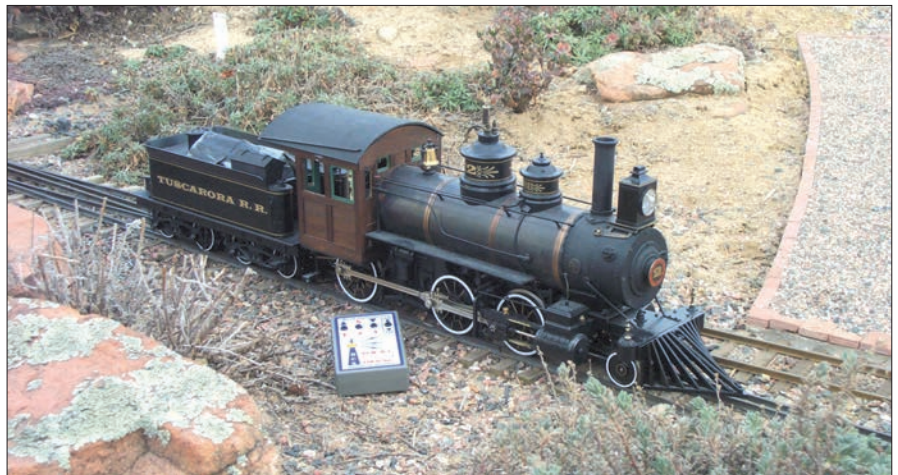
Radio control frees you from the vagaries of track power, but the R/C system must be purchased separately and installed, as it was in this engine.
