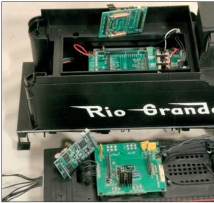
The top plug-and-play socket, in a Bachmann K-27 tender, is accessible by removing the coal load. Below it is an Aristo-Craft C-16, and its entire shell must be removed to gain access to the socket.
