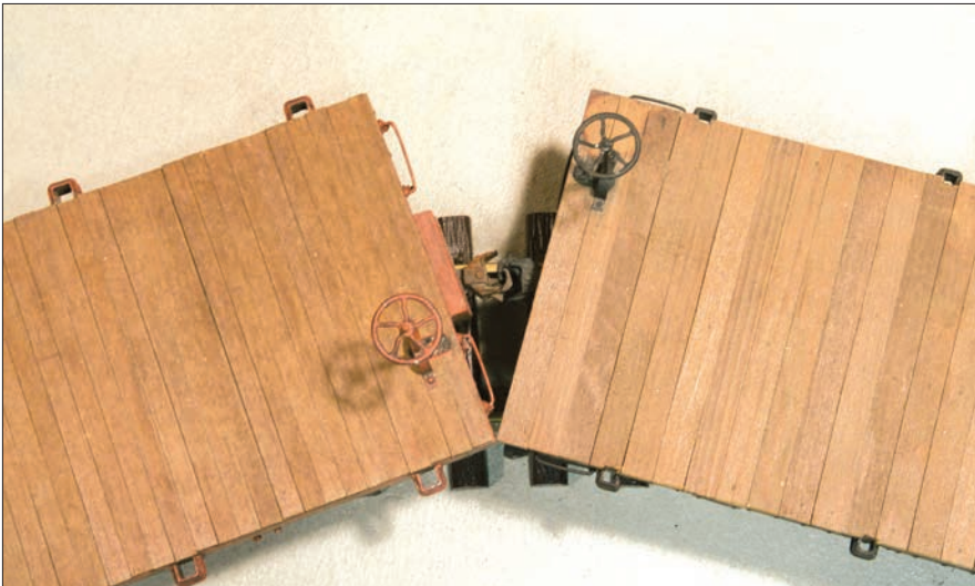
Wider-radius curves are needed for body-mounted couplers because they generally couple more closely, and the corners of the cars get in the way.
