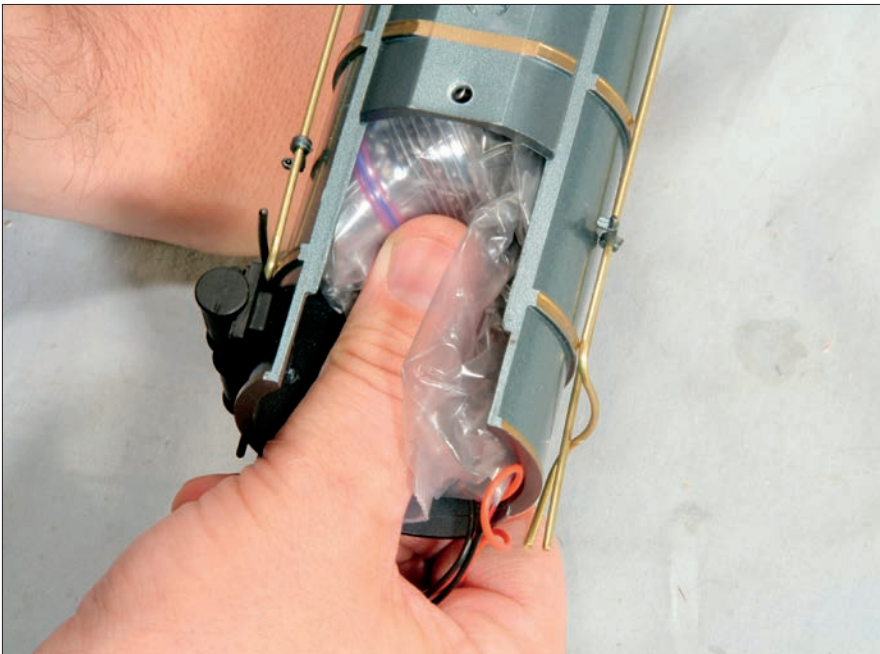
If you are able to remove the electronics from the boiler of a steam locomotive, then you can stuff in more weight. Here, I am placing a Ziploc bag full of shot into this boiler.
