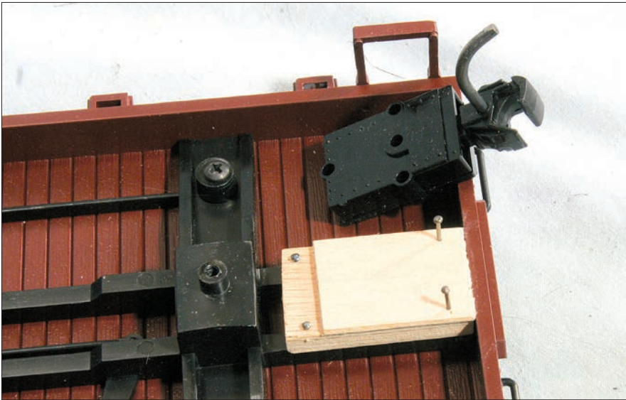
Many manufacturers' equipment has to have a suitable mounting surface built up with styrene or wood. The small pins are pushed into the plastic frame of the car to help hold the mounting pad in place once it's glued.
