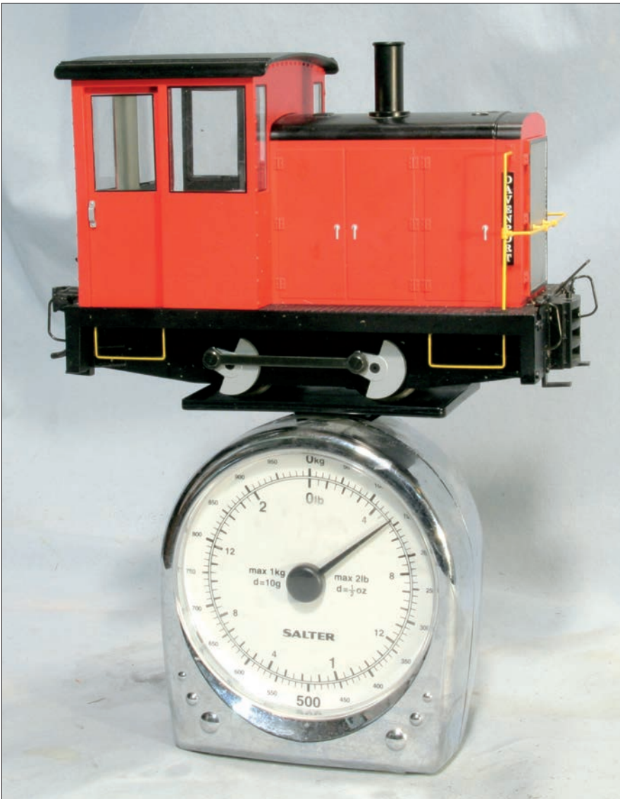
How much our locomotives weigh has a lot to do with how well they perform. The heavier they are, the more they'll be able to haul. But there's a trade-off. The more they weigh, the more stress it puts on the gears. Balancing the two is something of a guessing game.
