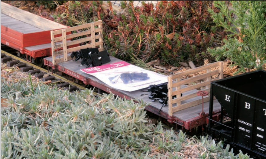
Couplers are perhaps the most important aspect of a train, as they constitute the hardware that allows the cars to stay together. I standardized mine with body-mounted Kadee couplers on my Tuscarora Railroad. Proper mounting is the key to reliable operation.
