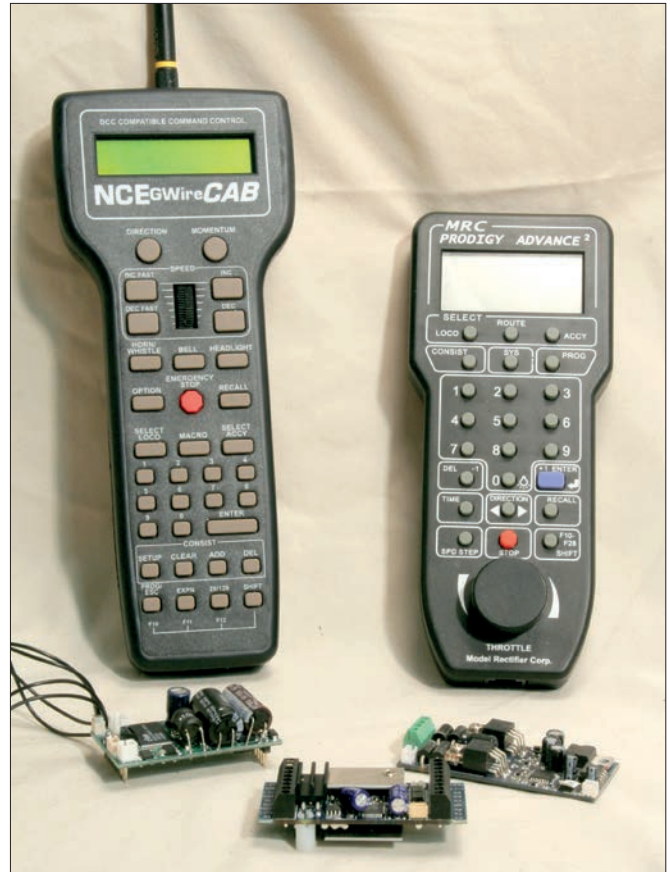
Open architecture DCC allows you to use any DCC controller with any DCC decoder. There may be subtle differences in how each works in terms of programming and controlling various functions, but they all work together. Shown are products by NCE (left) and MRC.
