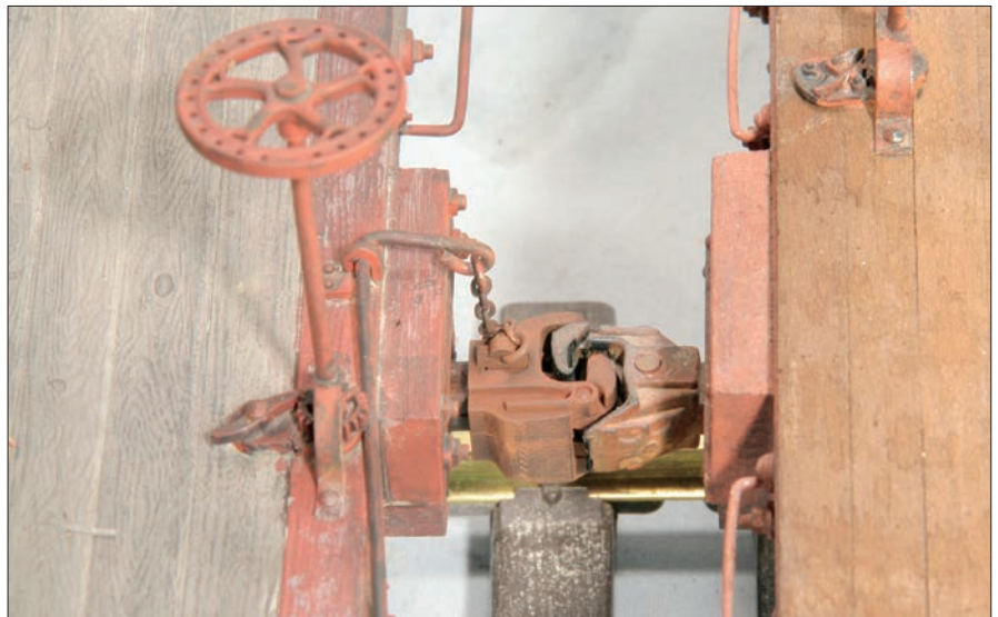
Some brands of couplers are compatible with Kadee (on right), such as this Accucraft 1:32 coupler (on left).
