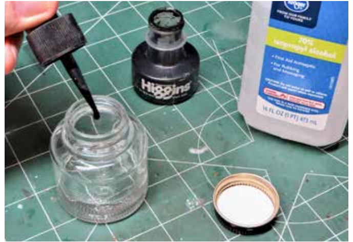
2 The classic solution. Bob added a few drops of Higgins waterproof India ink to a small glass jar of 70 percent isopropyl alcohol to produce the stain he used on the stripwood. He didn't want the stain too dark, as that could hide the wood grain.
