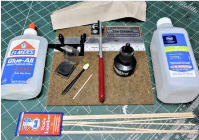
1 Tools of the trade. Here are the materials and tools Bob used for his flatcar deck project. Shown from top: sandpaper, white glue, black chalk, a sponge-tipped makeup applicator, a toothpick, The Chopper, India ink, 70 percent isopropyl alcohol, and HO scale 2 x 6 stripwood.
