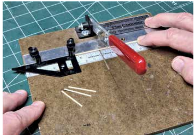
4 Quick cuts. Cutting 85 individual boards for each flatcar sounds daunting. To make the task more manageable, Bob used The Chopper from NorthWest Short Line. The plastic miter holds the wood to the same length for cutting.
