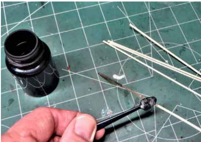
3 Adding variety. Bob used a sponge-tipped makeup applicator to pre-stain five of the 11 pieces of stripwood required for the project. He stained both sides the strips to minimize warping.
