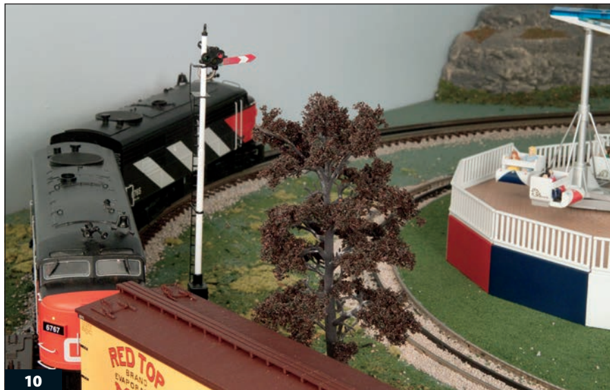
The passing train has activated this Lionel semaphore, dropping the arm and showing a red warning light.
