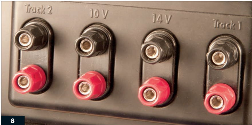
The power posts on this modern transformer are clearly identifiable by their red color.
