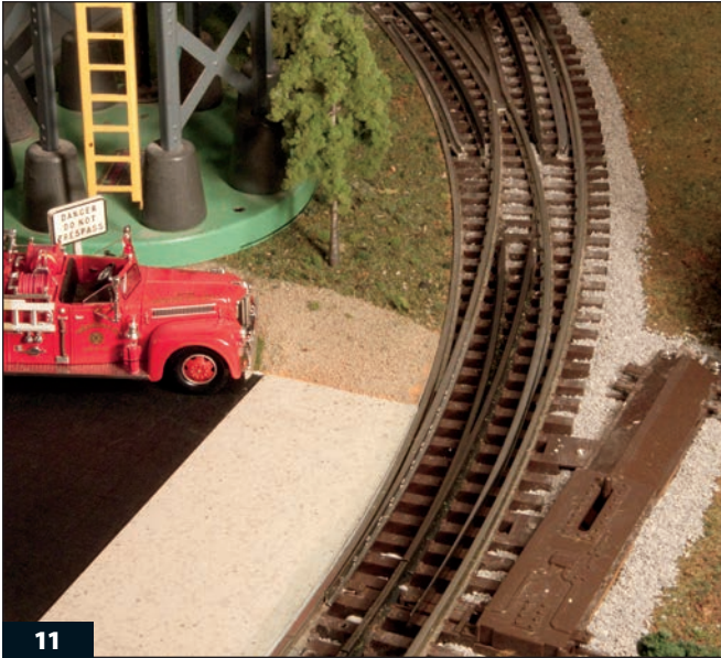
11 This Atlas curved 072/054 model is one of wide variety of specialty turnouts available with switch machines already installed.
