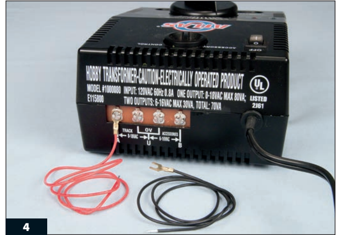
4 This Atlas starter-set transformer is easy to wire. The red wire goes to post A and the black wire to either of the U (ground) posts. It features a separate circuit for accessories (post B). Connections to the posts are easily made with the spade lugs on the end of the wires.
