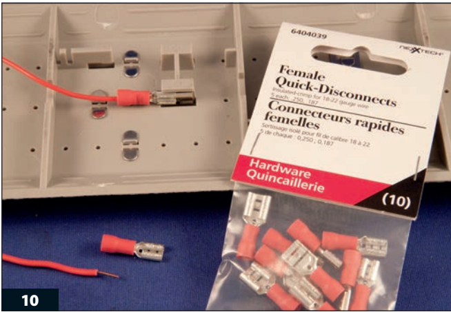
10 These packaged quick-disconnect female lugs are similar to the ones on a FasTrack system. Two size connectors are sometimes packaged together. The smaller size is the correct one to use with FasTrack.
