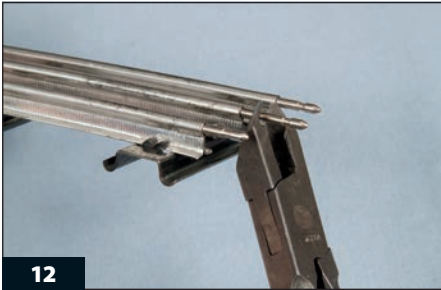
Plastic track pins replace the metal variety in the middle rail to create an insulated block.
