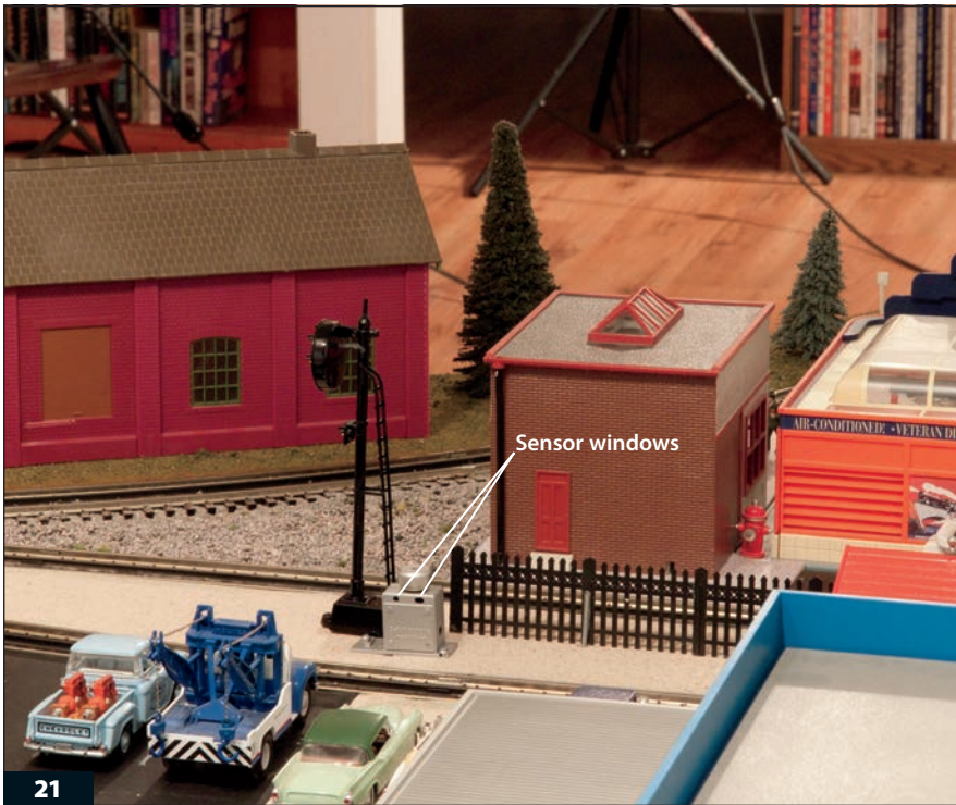
21 When positioning this infrared detector from Z-Stuff for Trains, the sensor windows must face the track in order to detect a passing train.
