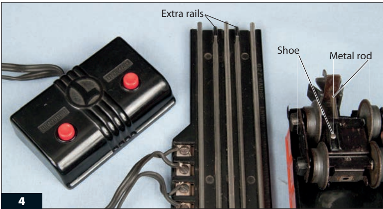
4 The first Lionel remote control operating cars were introduced shortly before World War II, along with an operating track section that provided hands-free uncoupling.
