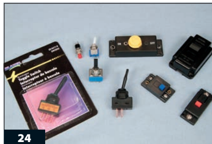
24 Toggle switches (left) and slide switches (right) are two types of switches that you may want to use for operating accessories on your toy train layout.
