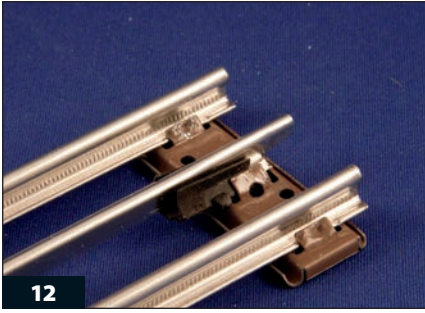
12 A loose or broken piece of insulation can allow the middle rail to touch the tie and cause a short circuit.
