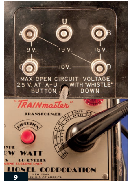
On the back of this Lionel RW Transformer (top), the letter U designates the throttle.
