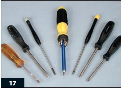
17 Flat-bladed (left) and Phillips-head screwdrivers (right) come in many sizes. The large screwdriver in the center has interchangeable ends of various sizes and types.
