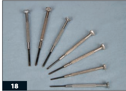
18 A variety of miniature screwdrivers are needed when working with today's sophisticated O gauge trains and accessories. They can be purchased economically in sets such as this one.
