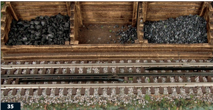
35 Atlas control rails are unobtrusive when installed in a section of ballasted track. They may also be installed on the ties of GarGraves and Ross track sections.
