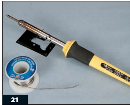
21 A 30-watt iron is adequate for most soldering tasks on a model railroad.
