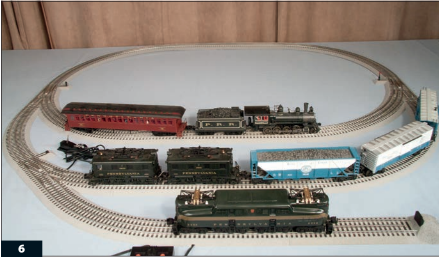
O gauge trains from different manufacturers are basically compatible and can be used together on the same layout no matter what brand of track you have. Coupler height and size, the amount of voltage needed to operate the motors, similar smoke units, compatible whistle and bell circuits, and identical wheel gauge are just some of the features that allow you to mix and match equipment.
