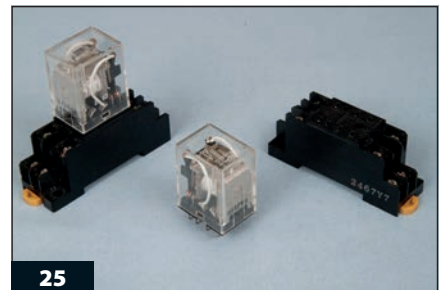
25 Electronic relays often come with convenient plug-in bases that provide screws for connecting wires.
