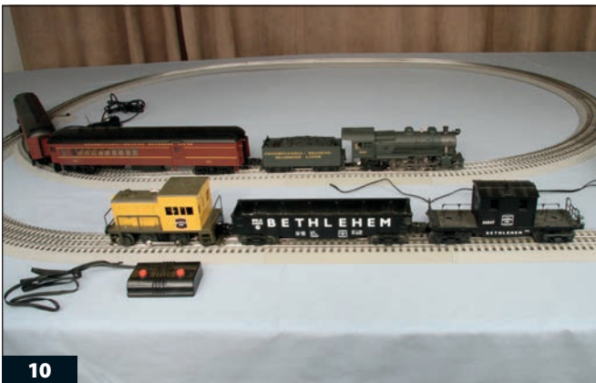
10 Two trains may operate independently on the same layout when the track is wired in blocks.
