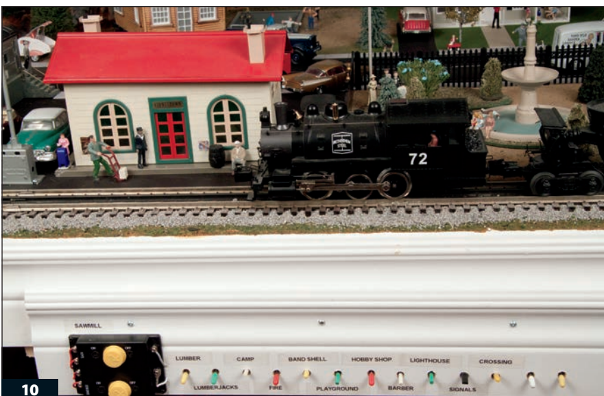
Grouping control switches in one area reduces the amount of wiring needed to connect them to the transformer.
