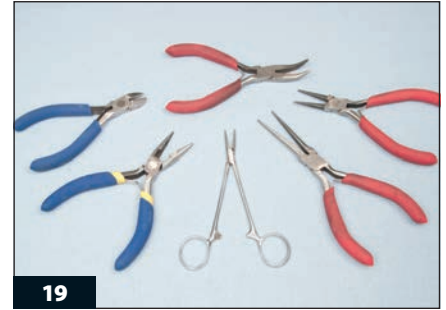
19 Specialized pliers perform a variety of tasks. In the center is a medical hemostat, useful for holding small parts securely. The pliers with the blue grips (top left) is a cutting tool that can be used to strip wires.
