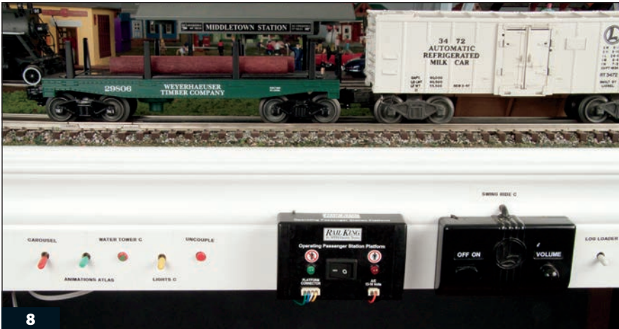
Sometimes dedicated control boxes work best with complex accessories, such as the MTH animated station controller and the Lionel controller for the musical swing ride. At left, in ¼" holes, are three miniature toggle switches and two push buttons that control various components. At right is the on/off switch for an American Flyer log loader.
