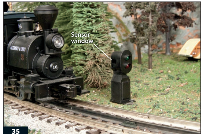
35 This Z-Stuff for Trains dwarf block signal contains an infrared detector, activated by the sensor window that faces the track.
