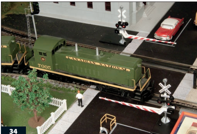
34 Z-Stuff for Trains crossing gates operate by optical detectors or with an insulated rail.
