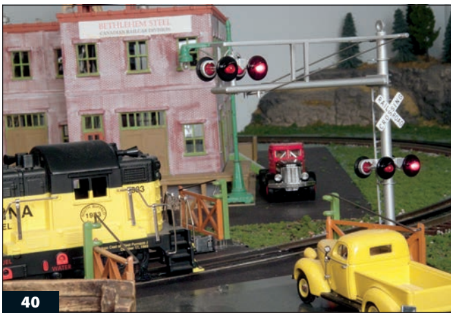
This MTH grade crossing signal contains an electronic circuit that flashes the red lights alternately at a realistic speed.
