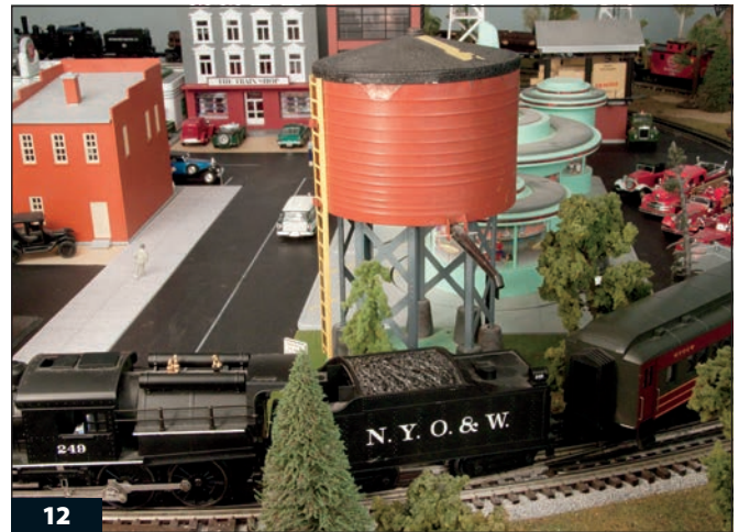
12 Filling the tender with water, pre- and postwar American Flyer style, takes place as a solenoid lowers the spout with the push of a button.
