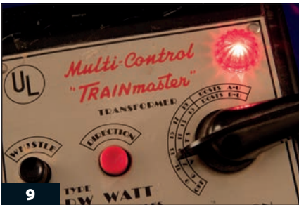
9 On a vintage transformer, a red overload light warns of a short circuit or an overload caused by having too many trains and accessories connected to the transformer.
