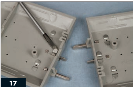
To insulate a FasTrack section, pry up the middle rail, remove the track pin, and replace the rail.
