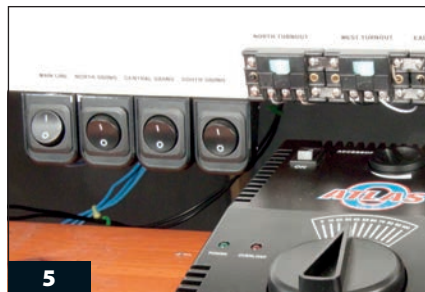
5 Four on/off rocker switches are labeled for the track blocks that they control. The one at left (the main line) is turned on. At right are controllers that came with Atlas turnouts.
