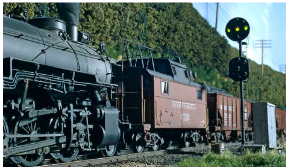
3. Working in helper service, an H10 Consolidation passes a PRR position-light signal. See the above illustration for information about these distinctive signals.
