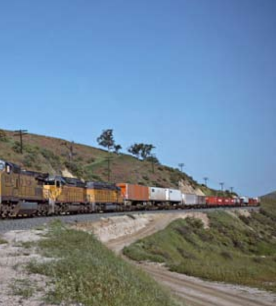
Don's track plan provides room for three- and four-unit consists of UP's huge fleet of C-C road locomotives. It isn't all for show as multiple units will be required to haul trains up the 2.4 percent grades. Photo by Ed Sarber
