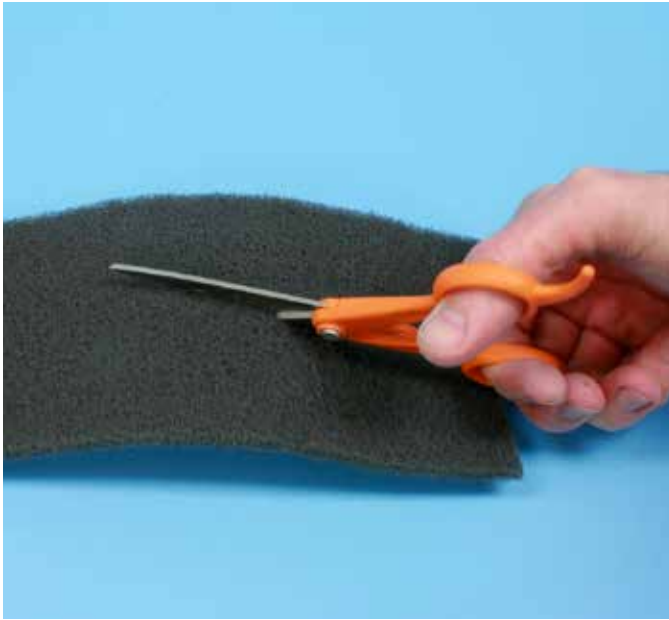
FIG. 2 Cut undulating shape. After cutting the continuous roll of scuff pad into 4-foot sections, use scissors to make a wavy, lengthwise cut down the middle of the strip.
