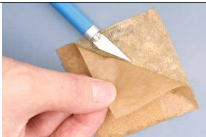
To simulate asphalt siding, Kathleen starts by soaking squares of 220-grit sandpaper overnight in solution of water and dish washing liquid. Then she separates the paper layer from the grit layer using a hobby knife.
