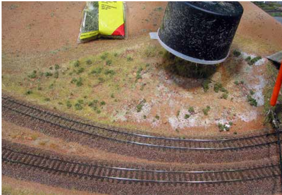
FIG. 2 STATIC GRASS. Horst uses an electrostatic applicator to apply grass fibers on diluted white glue. The ground wire of the applicator is at right.
