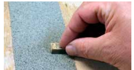
FIG. 4 TAMPING IT DOWN. Peeling up the tape leaves the edges of the road rough. Tom presses the edges into shape by hand, then uses a piece of basswood to tamp down the surface.
