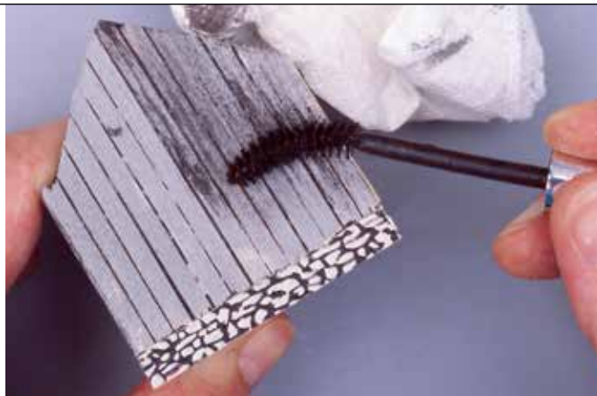
Kathleen uses the drybrush technique to apply mascara weathering to the siding. After wiping much of it off, she darkens random areas and lightly sands others.
