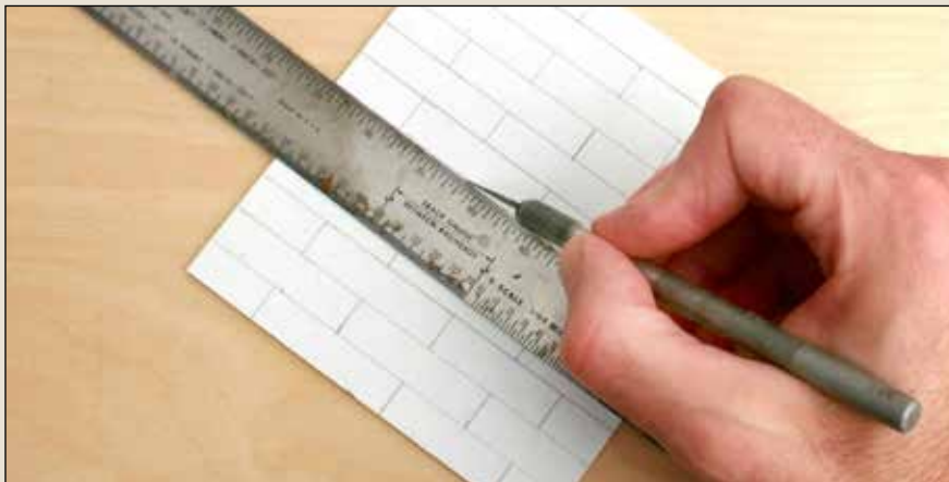
Lance uses a hobby knife to scribe lines on scale 3-foot centers, a typical width of a membrane panel. He then scribes lines to represent the scale length of a panel between 12 and 20 feet.
