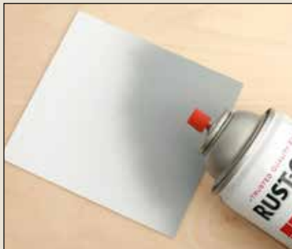
To keep the stark white styrene surface from showing through, Lance first paints the roof gray.
