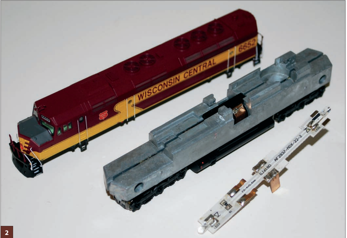
Here's an Athearn N scale FP45 with its original lighting-circuit board removed.
