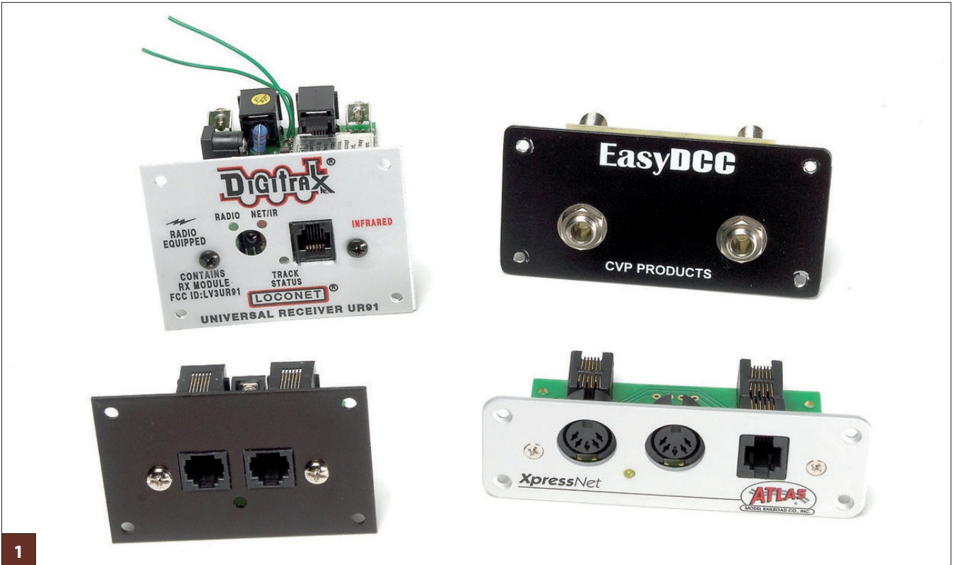
Throttle panels clockwise from upper left include a Digitrax radio panel with six-pin RJ tether port, an Easy DCC panel with two 1/4" audio jacks, an Atlas (Lenz) panel with two DIN sockets and a six-pin RJ jack, and an NCE universal panel with two four-pin RJ jacks.
