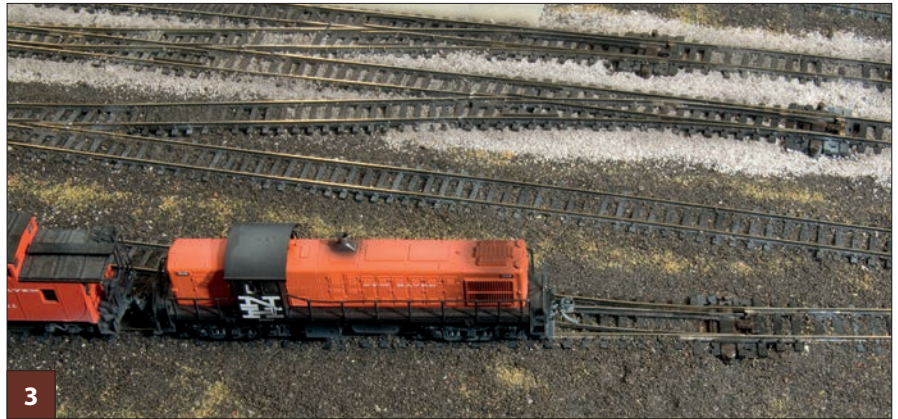
This locomotive has just caused a short circuit by running into an open turnout—note that the points are thrown for the other route. This is the most common cause of short circuits.
