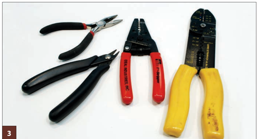
Good-quality pliers, wire cutters, and a wire stripper are essential tools for installing wiring.
