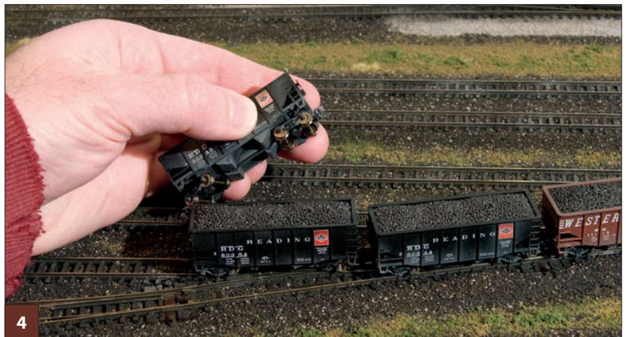
Derailments—especially at turnouts and crossings—can cause short circuits when the involved cars have metal wheels, as on these N scale hoppers.
