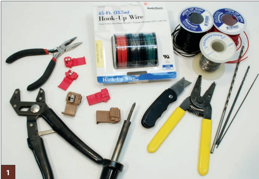
1 Wiring tools include a soldering iron and resin-core solder, pliers, wire cutters, and wire strippers. The brown and red suitcase connectors allow for solderless wire connections. Wire comes in different colors and gauges.
