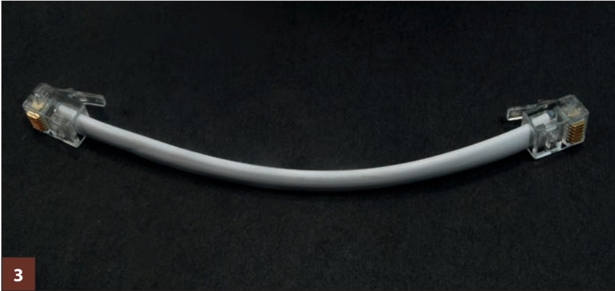
Phone cables can be made in two different ways. Note that with the cable flat, the plastic tabs on the connectors are both “up.” This indicates pin 1 is connected to pin 6. This style of cable is not generally used.
