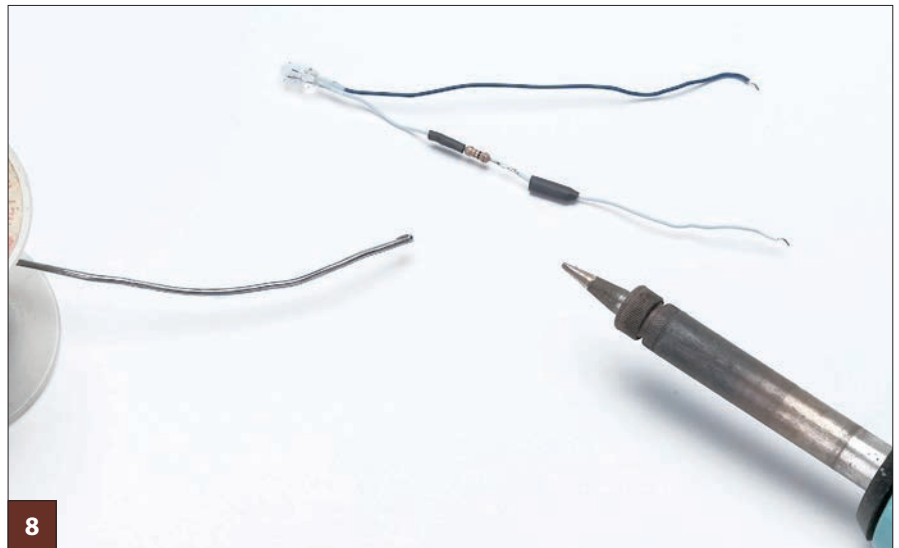
A resistor must be wired in series with 1.5-volt bulbs to work with decoder lighting output functions.
