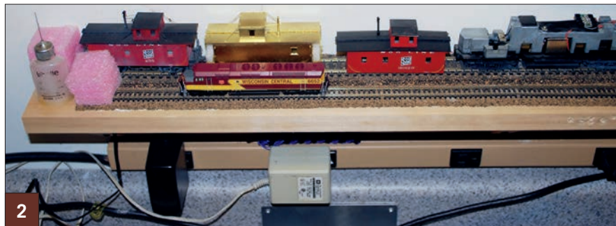
2 Test track. Before and after installing a decoder, I try out locomotives on a test track. I have both an HO scale track for my Soo Line layout and an N scale track for my son's Wisconsin Central model railroad.
