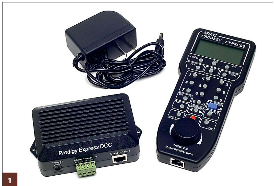
MRC's Prodigy Express is an example of a basic DCC system with lots of features. It includes a throttle (right), command station/booster (left), and power supply (top).
