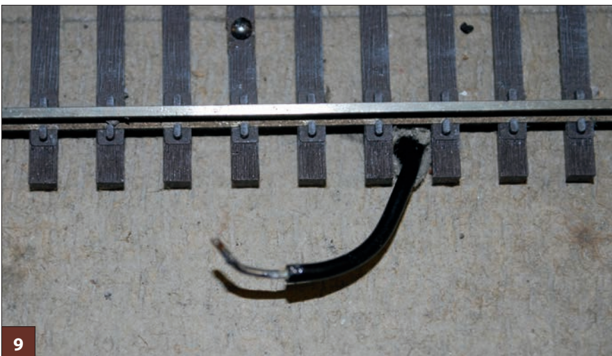
Insert and tin the end of the feeder wire. Putting a slight bend in the wire will allow it to fit snugly against the web of the rail.
