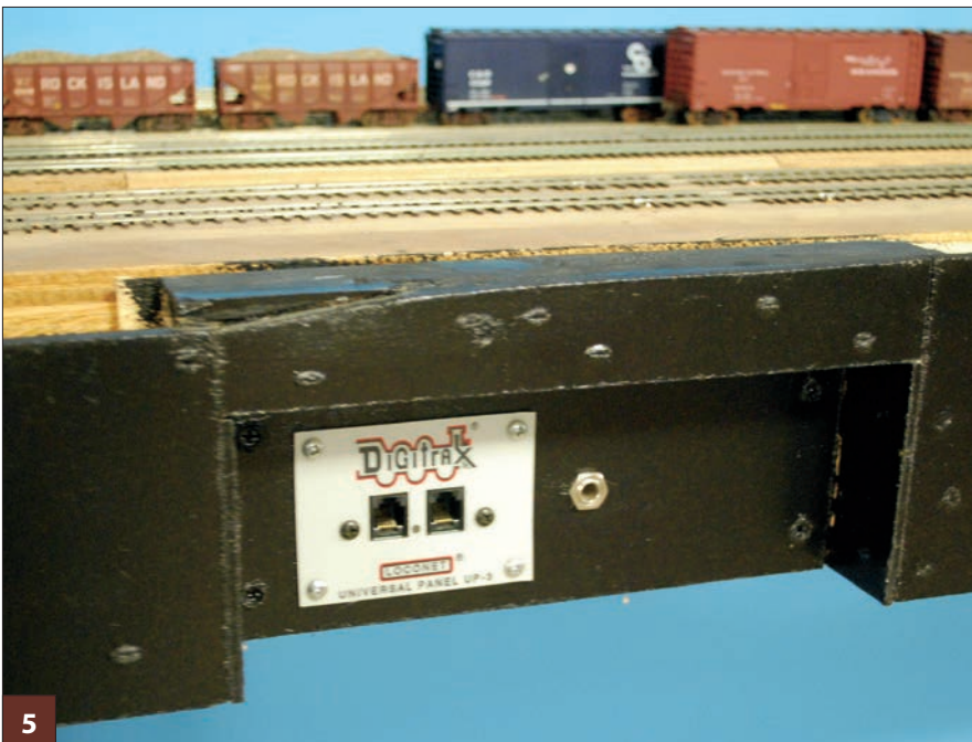
Here’s a standard Digitrax throttle panel, with two jacks, installed on the fascia of Bob Perrin’s HO scale Illinois Central layout.
