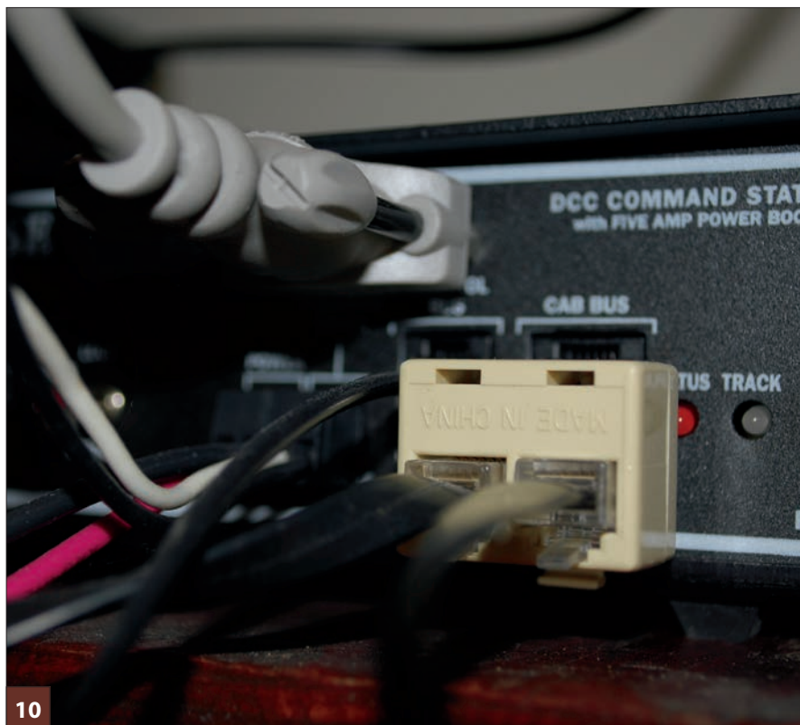
I used a commercial six-conductor phone cable splitter to "tee" the cab bus right at the command station.
