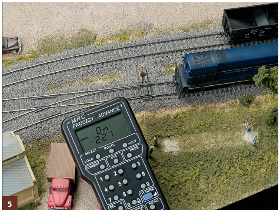
Stationary decoders allow operators to control turnouts with their throttles. Both the switch machine and decoder are mounted below the layout.
