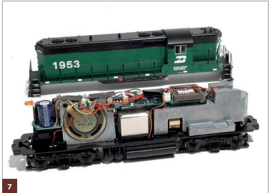
7 Many locomotive models are available with DCC decoders already installed. This HO scale Proto 2000 GP9 has a factory-installed QSI sound system with speaker.
