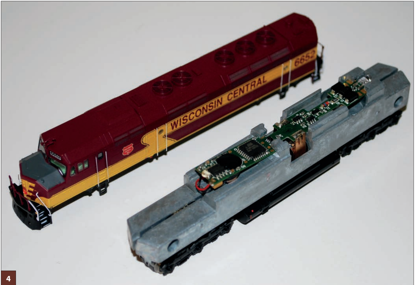
The MRC sound decoder is an easy drop-in installation in the FP45.
