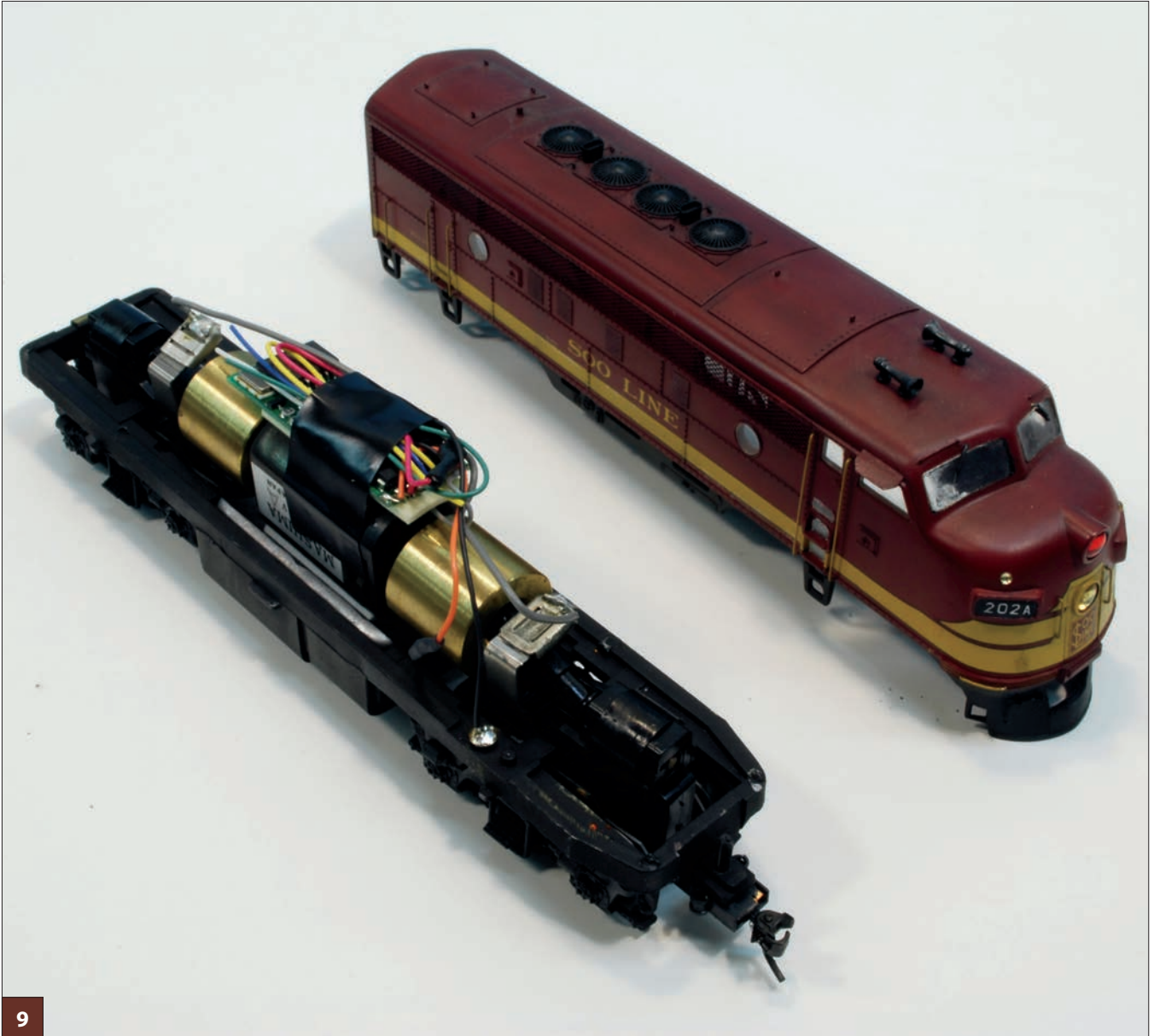
This is an older HO Athearn standard locomotive that has been repowered with a can motor.
