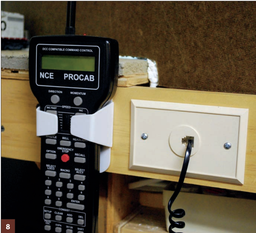
At the end of my cab bus, I use a commercial phone jack as a throttle panel rather than one specifically made for DCC. Only one plug-in is needed here.
