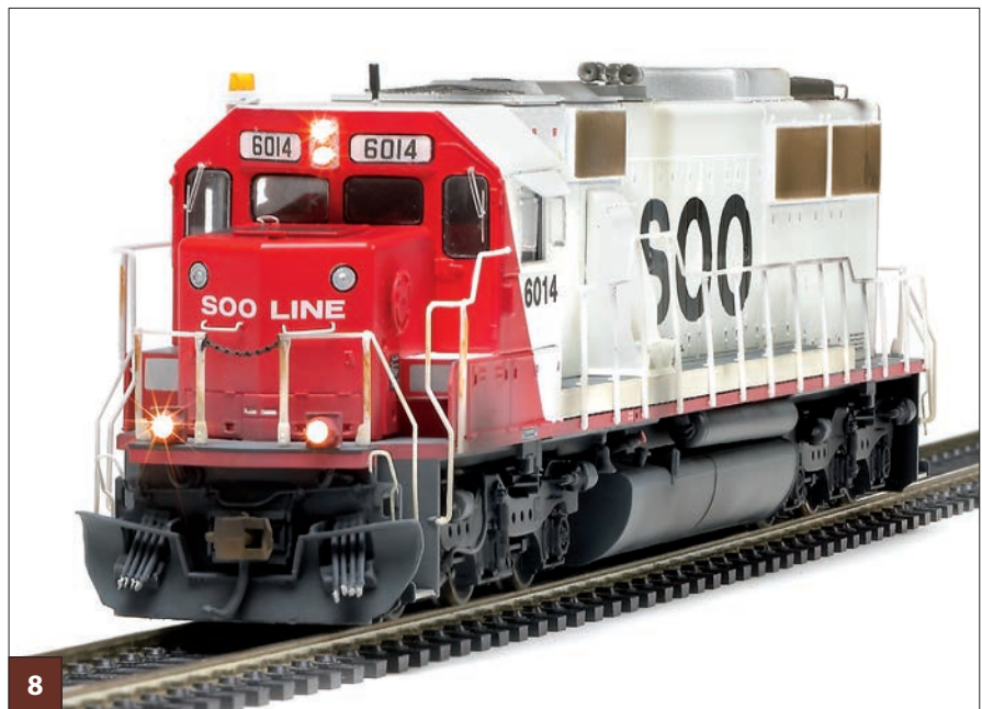
8 Along with motor control, decoders have extra outputs called functions. These are being used to control headlights, ditchlights, and a rooftop beacon on this HO scale SD40.
