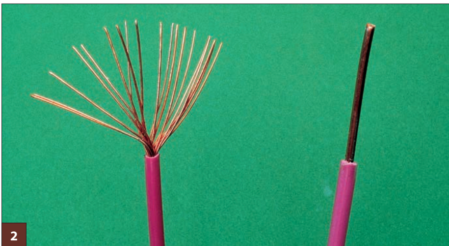
2 Wire is either stranded (left) or solid. Stranded wire is more flexible than solid.
