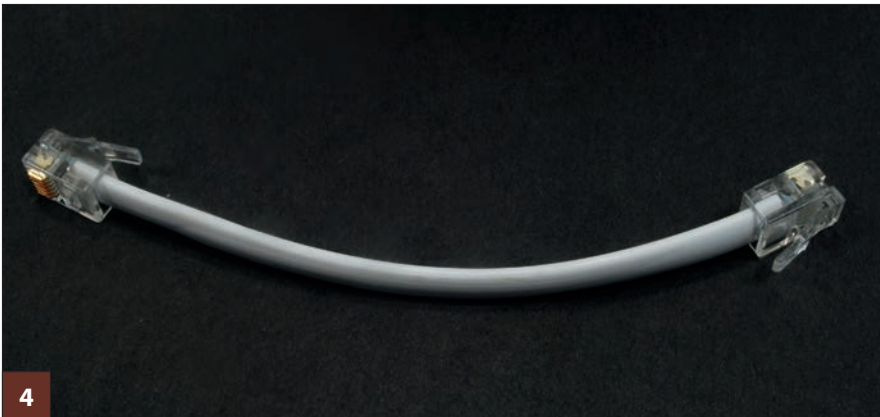
The most common design for phone cables is with one tab pointing up and the other down. This connects pin 1 of one connector to pin 1 of the other connector. This is how most DCC cab bus cables should be wired.
