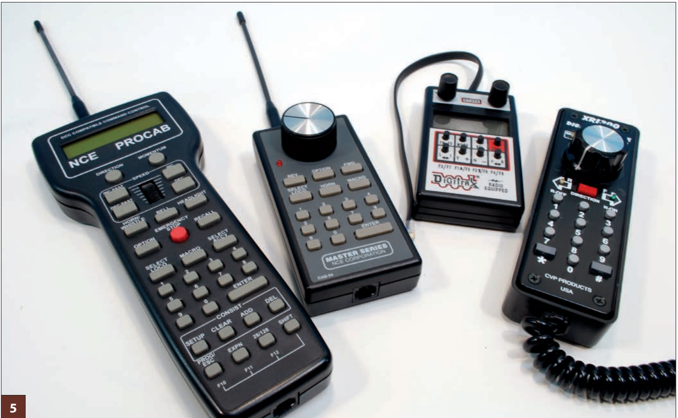
There are many styles of DCC throttles. Make sure the system you purchase has a style of throttle with which you are comfortable. From left to right are an NCE Procab, Cab O4PR wireless for NCE's Powerhouse Pro, a Digitrax wireless, and an Easy DCC (CVP) tethered cab.
