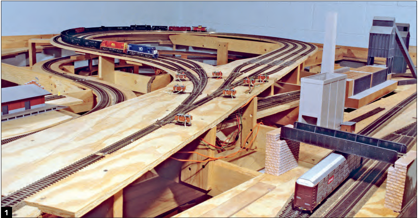
On the HO scale Ohio Southern layout, three Peco curved turnouts are used to fit in a reverse loop staging yard. The switch machines are top mounted for easier maintenance and clearance underneath.
