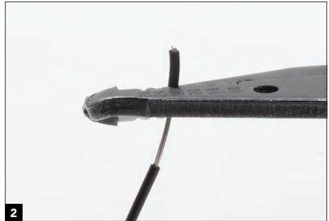
2 Use a pair of wire strippers to remove a short piece of casing on the 22 gauge wire.
