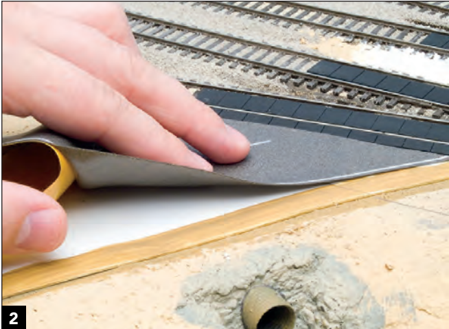
2 I put down .040" styrene sheet as a smooth base to provide good adhesion for the Busch foam asphalt highway material, which has a peel-and-stick back.
