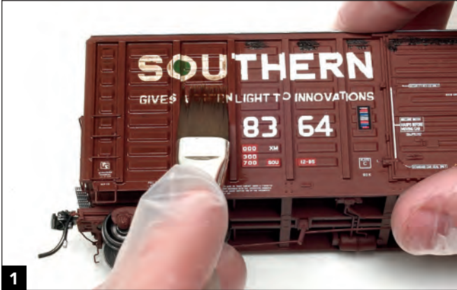
1 I used Turpenoid and Burnt Umber oil paint to give the boxcar a weathering wash. Keep the brush parallel with the exterior posts.
