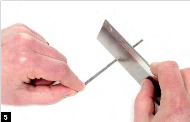
5 The plastic poles have molded wood grain detail, but to give them more of a rough texture, I scraped the poles with a fine-tooth razor saw.
