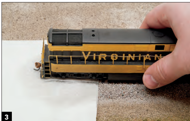
3 After just a few seconds of running, the towel picks up a lot of dirt and gunk that impede a locomotive's ability to run smoothly.
