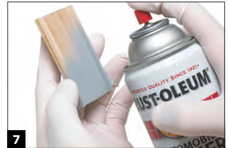
7 Keep a scuff pad handy to remove any fuzz from the wood before spraying it with primer.
