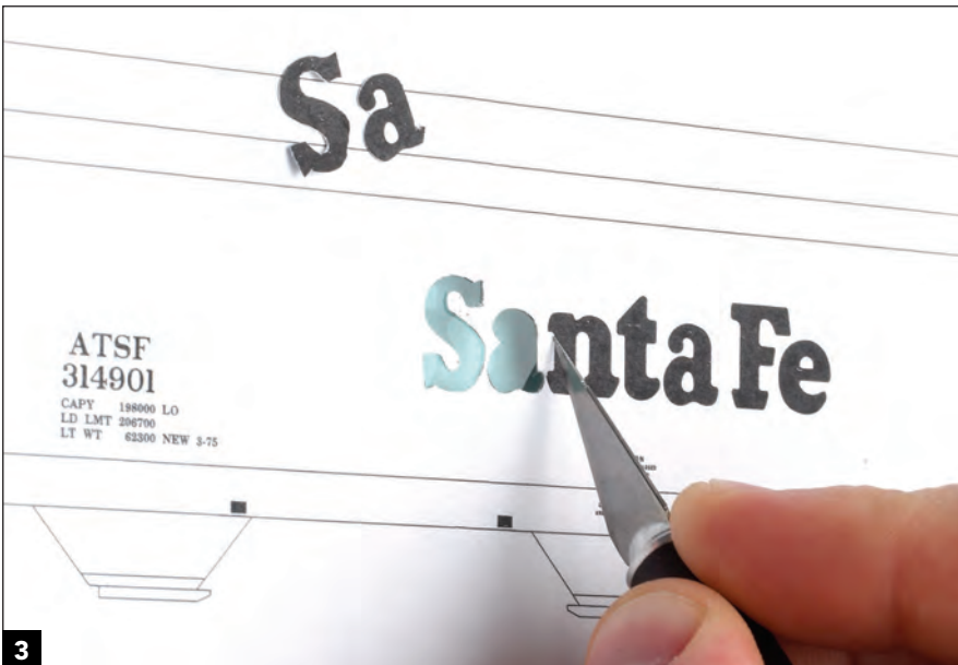
To make the stencils, I photocopied the decal-placement guide included with the Microscale set. I placed the paper on a piece of plate glass and used a hobby knife with a sharp no. 11 blade to cut out the letters.
