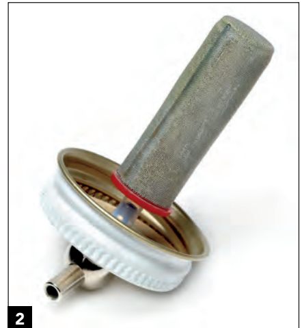
2 Dried paint and pigment clumps can clog an airbrush or ruin the finish on a model. This filter, sold by Micro-Mark, attaches to the siphon tube and keeps contaminants out of the paint stream.
