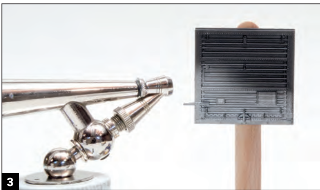
3 I also painted the doors Flat Aluminum. This made it easier to see the spray pattern and paint coverage while I airbrushed the doors with Steam Power Black.
