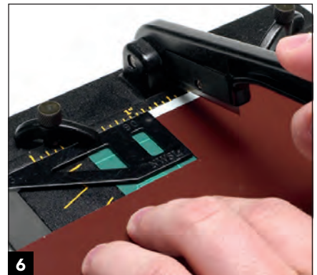
6 For crisp square edges on your trim film, cut it with a cutting tool having a fresh blade.
