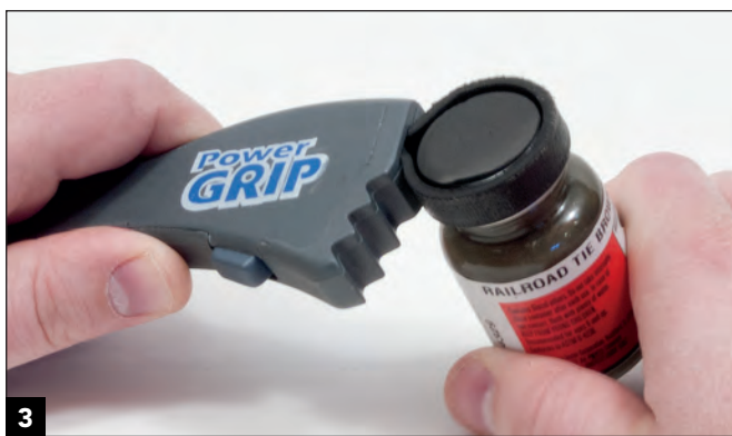
While more commonly used in automotive and plumbing repair, a strap wrench can also be used to remove a stuck paint bottle cap.
