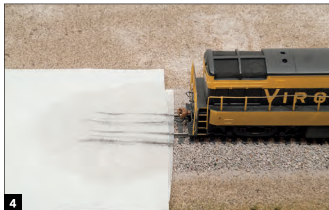
4 Offset the wet towel and repeat the process for the rear truck. Then run the wheelsets over a dry towel when you're finished.
