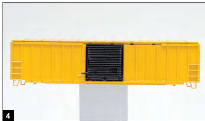
4 After I applied Polly Scale Clear Gloss and let it dry, the model was ready for decals and weathering.
