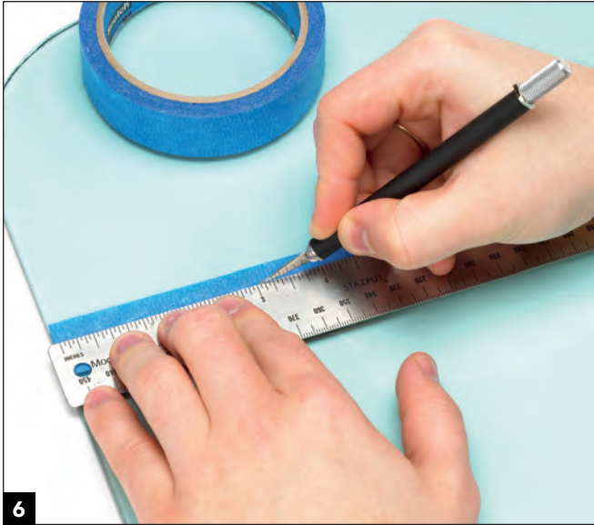
6 A favorite modeler's trick is to put masking tape on a piece of glass, lay a steel straightedge over it, and cut a strip using a hobby knife with a fresh no. 11 blade. Use the cut edge to mask the separation line between colors.
