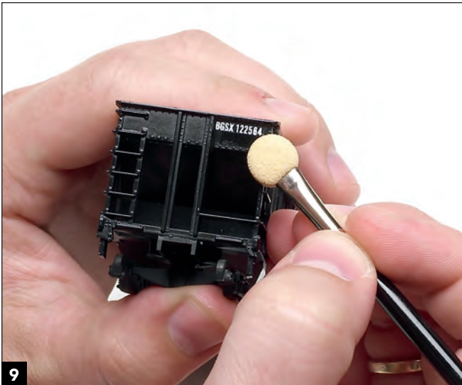
9 When the decals in position, use a sponge applicator to blot away excess water instead of cotton swabs or paper towels, which can leave lint on the model.
