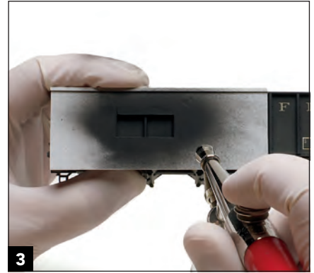
3 Set the air compressor at 20–25 psi, and apply the paint carefully in multiple layers, so it doesn't seep under the mask.
