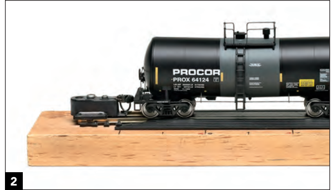
2 This test fixture makes it easy to quickly check coupler height and make sure they align. It also helps check the position of uncoupling pins on freight cars.
