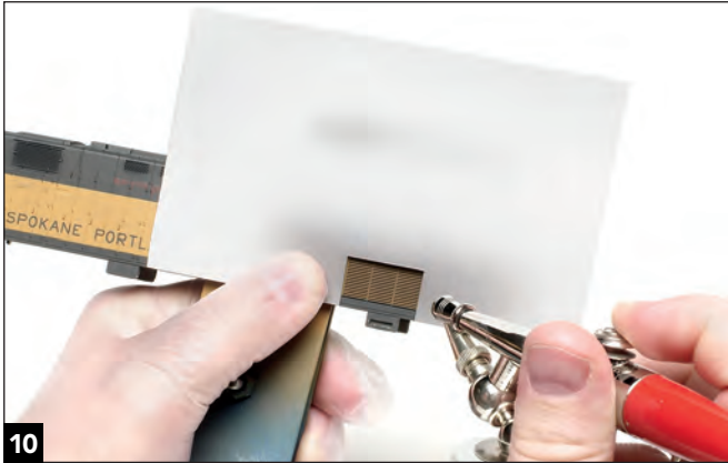
10 While airbrushing the radiator shutters, hold the mask in place with your thumb or use painter's masking tape.
