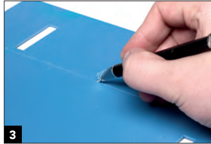
3 Using the back edge of the blade helps speed up the scoring process.
