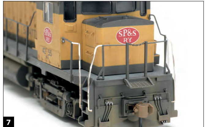
On the pilot, paint the connections on the m.u. cables silver and spray the bottom as done on the sideframes.
