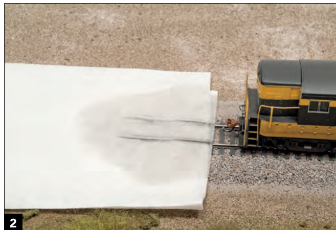
2 Place a paper towel over the tracks and wet it (but don't soak it) with isopropyl alcohol. Let the model start running, and then hold it in place and let the wheels spin for a few seconds.
