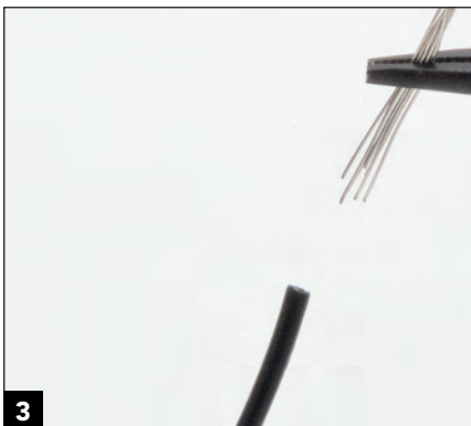
3 With the wire exposed, gently pull it out of the casing with needle-nose pliers.
