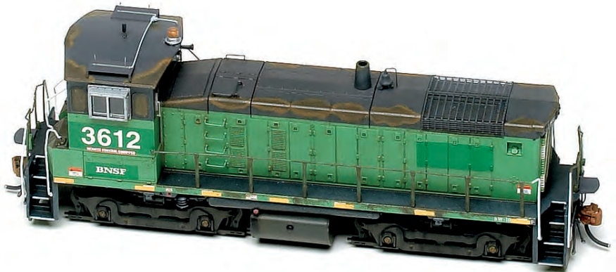
I used foam-tipped cosmetic applicators to simulate rust and paint wear on this Athearn HO scale BNSF Ry. SW1000 diesel locomotive.
