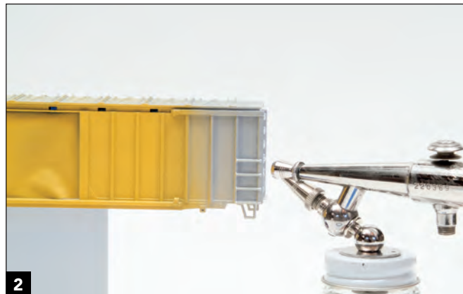
2 An even coat of Polly Scale Flat Aluminum ensures the yellow will cover evenly in just two or three coats. Fewer coats of paint makes it easier to preserve the model's fine details.
