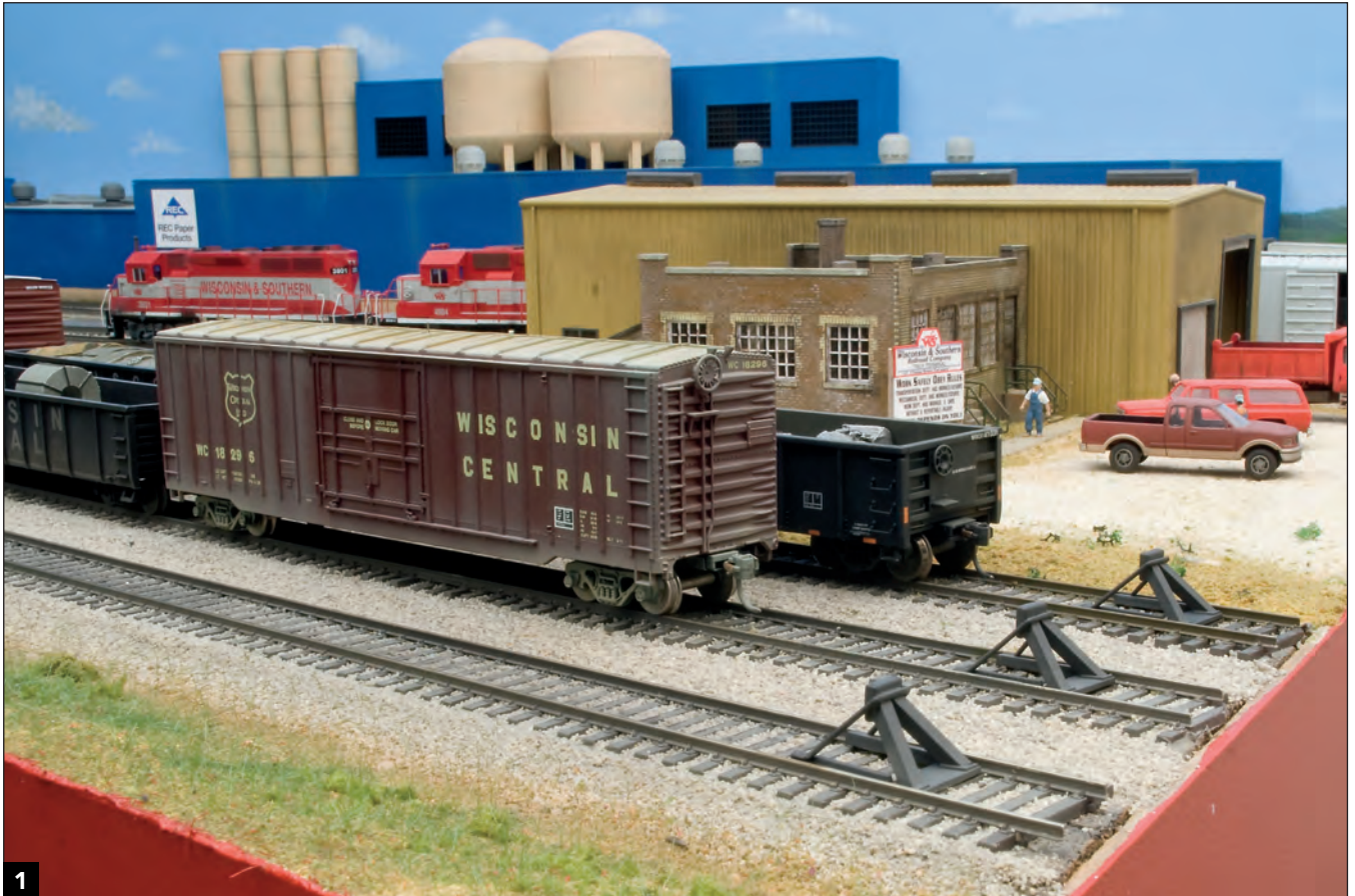
These Walthers HO scale bumping posts keep cars from rolling off the end of the rails on Model Railroader's Wisconsin & Southern's Troy Yard.
