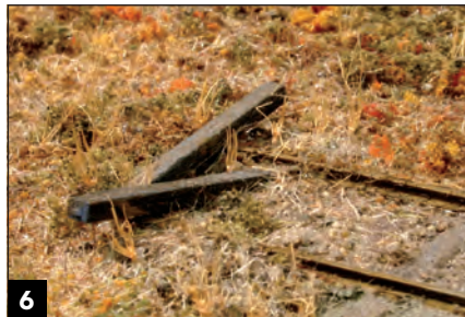
6 A simple and inexpensive wheel stop made of cross ties keeps slow-moving cars from rolling off the rails.
