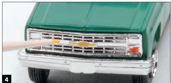
4 The grill on this model also features Chevy's trademark Bowtie. I used yellow-tinted Kristal Klear to fill in the ornament.
