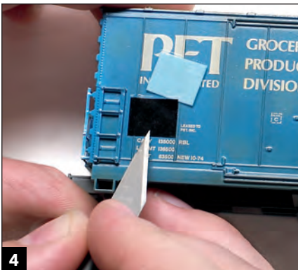
4 On this blue PET Inc. boxcar, I used black patches from a Tangent Scale Models decal set as a background for the restenciled white numbers and letters.
