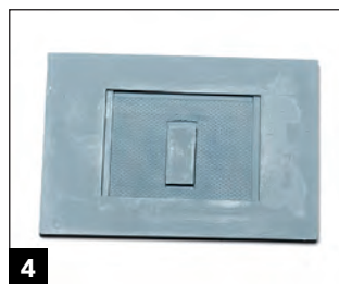
4 After the rubber hardened, I removed the mold from the box.
