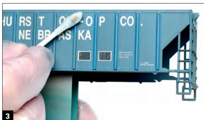
3 With the paint still fresh, I used a cotton swab dipped in Windex to remove the weathering coat from the face of each exterior post. Do this carefully so the swab doesn't remove paint from the body panels.
