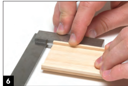
6 To re-create the lip between the curb and bridge deck, attach \frac{1}{8} " x \frac{1}{8} " stripwood with CA.
