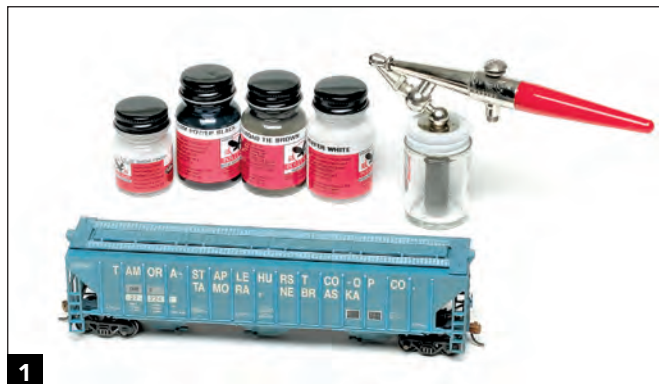
1 You can easily give your freight cars a general coat of grime with an airbrush and thinned acrylic paint.
