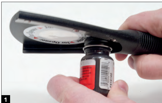
The Oxo jar opener has metal teeth which makes it easy to remove stuck paint jar caps. Use these with care, though, as the teeth can rip metal caps.
