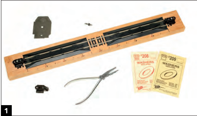
1 Useful tools for tuning up rolling stock include a coupler test fixture, truck tuner, NMRA Standards Gauge, height gauge, and a trip pin pliers.
