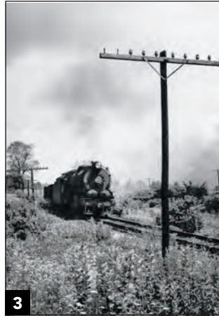
3 On this branch line of the Pennsylvania RR, the line poles were configured with single 10-pin crossarms.
