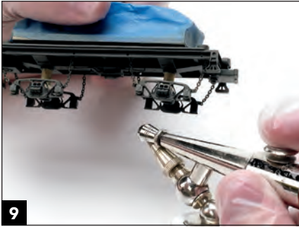
9 I separated the tender from the underframe and removed the wheelsets from the trucks. Then I sprayed the underframe with Polly Scale Dirt.
