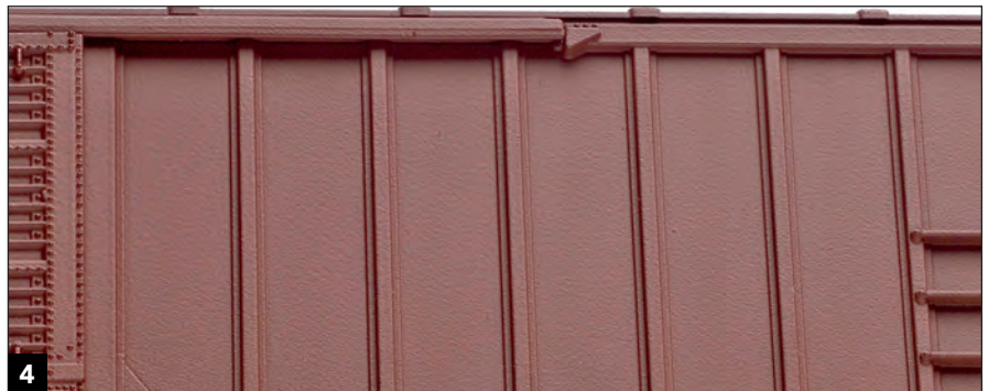
4 Rough finishes not only look bad, but they make it difficult to add decals. During painting, the airbrush was held too far away from this boxcar, causing the paint to dry before it hit the model.
