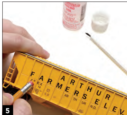
5 To remove the original lettering on a car when using a light-colored trim film, brush Micro Sol over the lettering and use a pencil eraser to take off the lettering.
